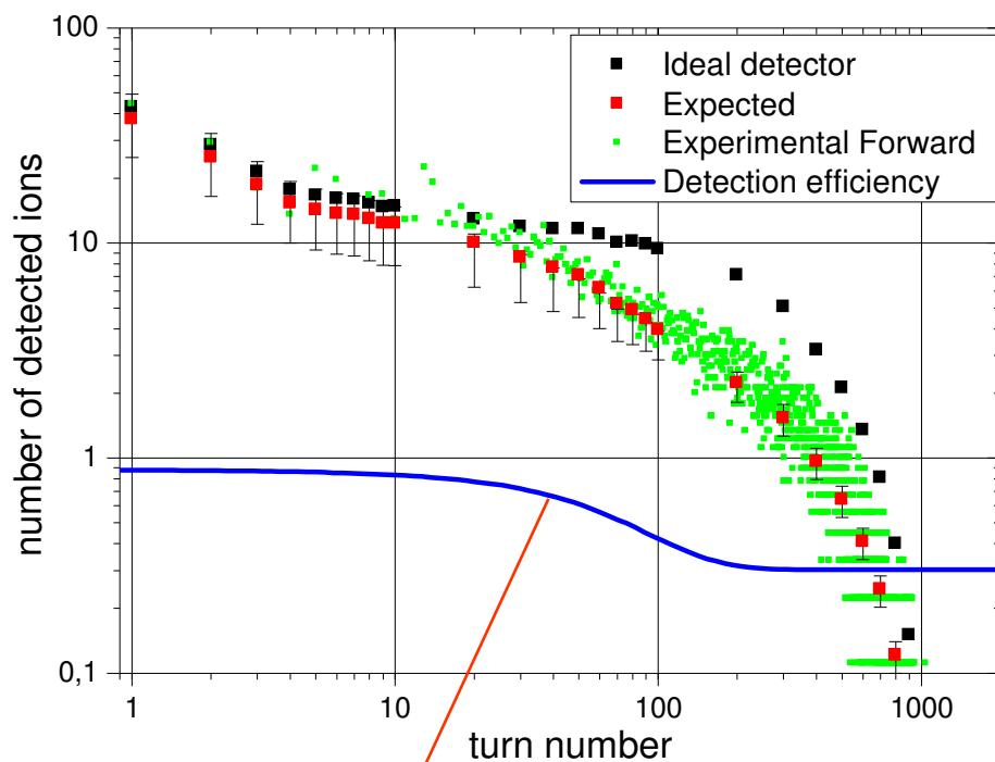
High rate limits detection efficiency
