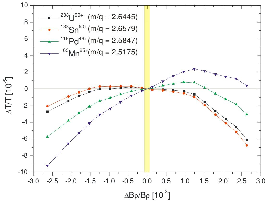
The isochronous condition can be fulfilled only for a small area
