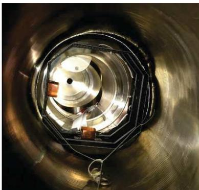
Figure 2: Two under 90 degree mounted Raspberry Pi cameras, directly installed into the toroid vacuum chamber. Kapton foil for protection of the cameras against particle impact and pulling rope for longitudinal mobility.
