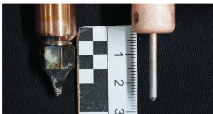
Figure 2: W80Cu20 tip (left), pure W tip (right) after approx. 20 ignitions with  $I < 50A$ ,  $t < 20ms$  per shot
