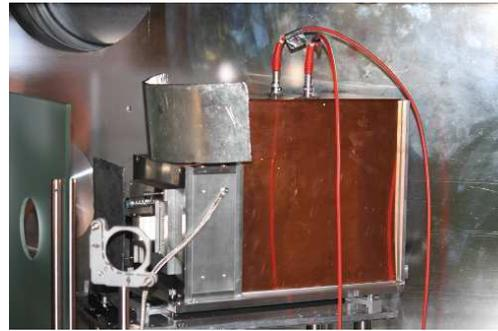
Figure 1: The new Thomson parabola inside the PHELIX target chamber.
