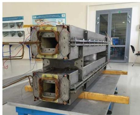
Fig.2. The first serial “twin” dipole for the Collider
