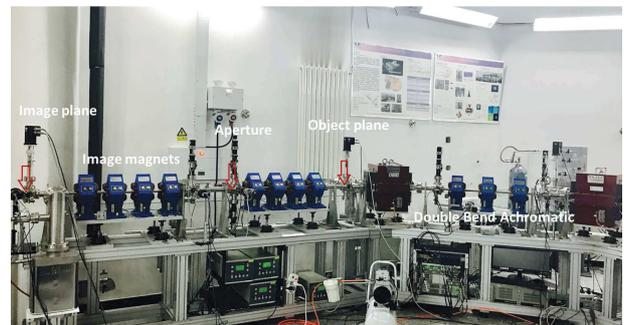
Figure 2: Newly constructed HEER beam line at THU, which is developed by IMP, THU and ANL together
