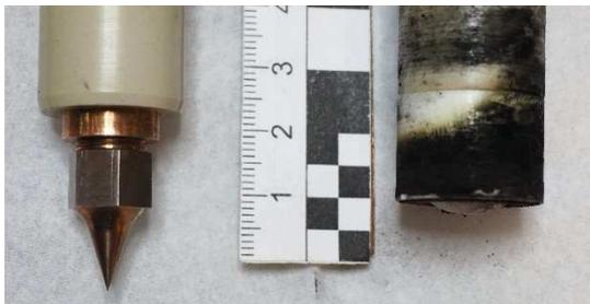
Figure 1: Unused Cathode (left) used cathode (left) with additional isolator (white). The cathodes are aligned such that the tips would be on the same height.
