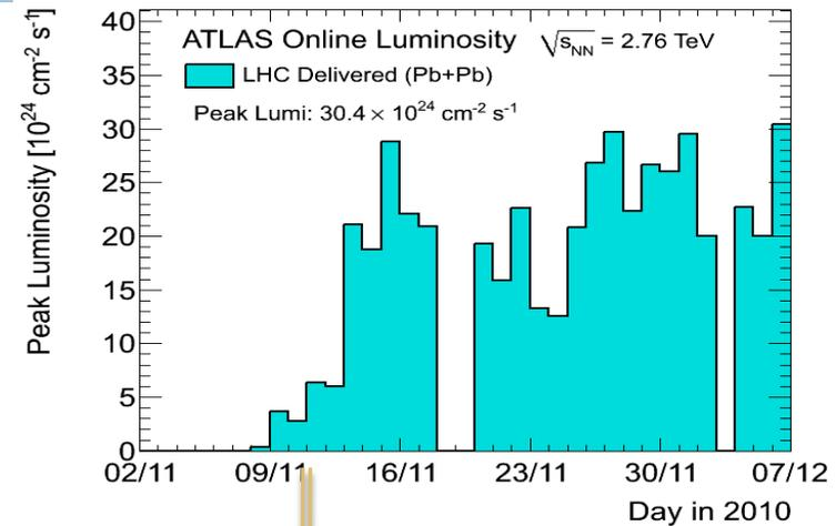
Only LVL1 trigger      Above  $5 \times 10^{24} \text{ cm}^{-2} \text{ s}^{-1}$  High Level Trigger (HLT) applied to filter out beam backgrounds and improve event selection. No selection based on physics objects like jets, muons, etc .
