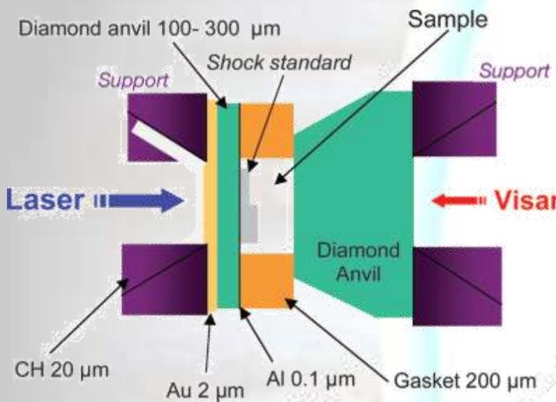
→ Laser-induced shockwaves in pre-compressed materials
