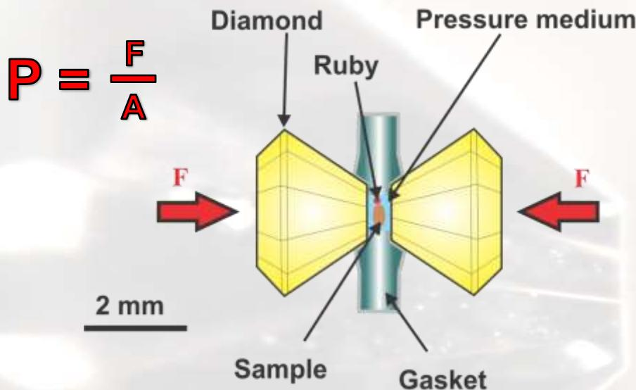
$$1 \text{ GPa} = 10 \text{ kbar} = 100 \text{ Kg/mm}^2$$
