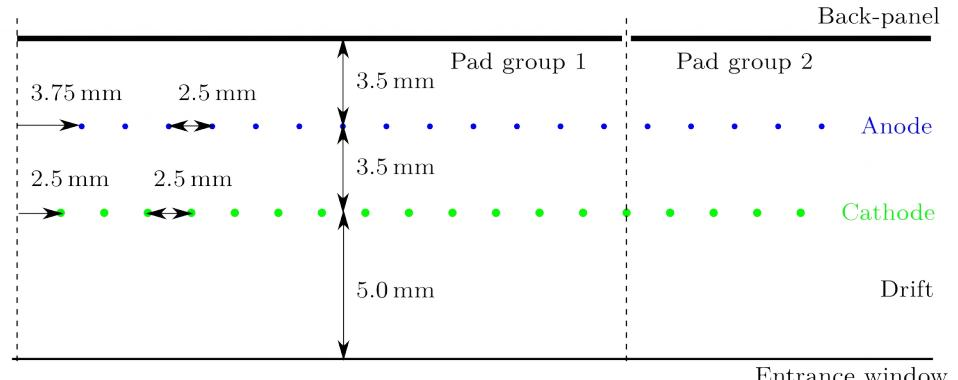
Favoured Anode+Drift HV geometry
