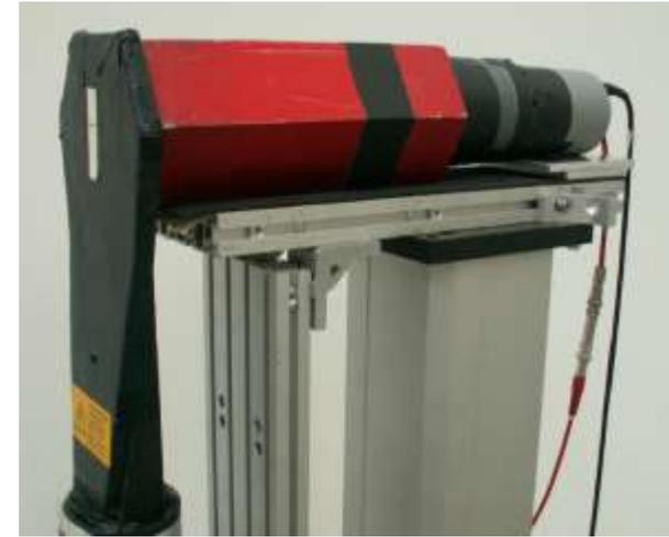
The  $\Delta E$ -E telescope detector
