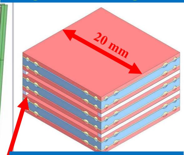
Six 250 µm gaps chamber composed of 3 double gap "sandwich" chambers of each two  $Al_2O_3$  electrodes and one SiC/Si<sub>3</sub>N<sub>4</sub> resistive electrode
