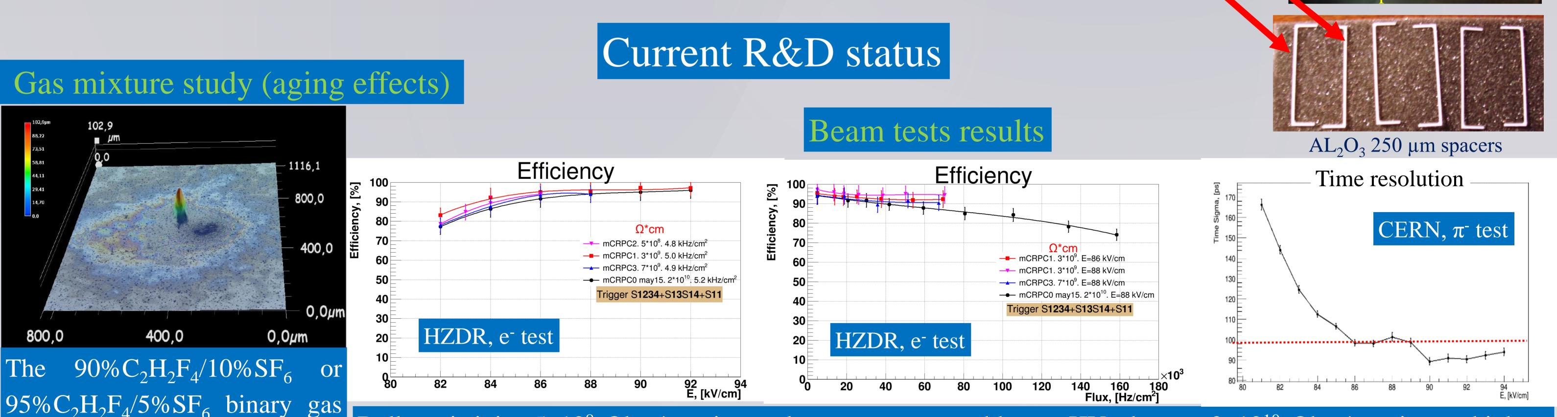
Bulk resistivity 5x10<sup>8</sup> Ohm\*cm is too low to operate stably at HV plateau; 2x10<sup>10</sup> Ohm\*cm is too high to operate at rates higher than 100 kHz/cm<sup>2</sup>. Efficiency (~96-98%) and time resolution (~80-90 ps) are consistent with expectation. MAXIM 3760 preamplifier was used, for comparison with ALICE R&D data.
