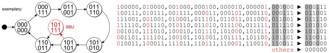
**Figure 2.23:** Depiction of SBU impact on the state transition diagram of a Hamming distance  $d=3$  encoded FSM. The EDAC feature enables reliable detection of the upset condition and therefore allows continuation of operation without undefined states or transitions while eliminating the necessity of an FSM reset. This EDAC scheme works even without a Hamming decoder when auxiliary states are added to the logic design [442].
