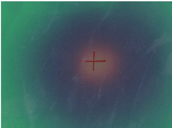
**Figure 5.3:** Sample picture for a radiation sensitive radiochromic film (GAFCHROMIC EBT by ISP) used for alignment purposes within the beam line. The picture has been taken during proton irradiation on August 5th, 2014 at COSY in Jülich, Germany.
