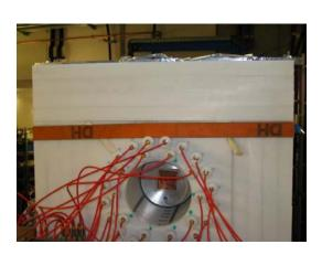
The Beta dELayEd Neutron (BELEN) detector, based in <sup>3</sup>He counters embedded in a polyethylene matrix, located around Silicon IMplantation Beta Absorber (SIMBA).
