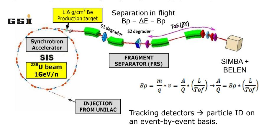
The detection system is based on a stack of SSSD- and DSSD-detectors for measuring ion-implants and beta-decays (SIMBA). Implants-region was surrounded by the 4n neutron detector BELEN.
