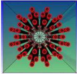
Use BELEN to measure beta-delayed neutron emission
