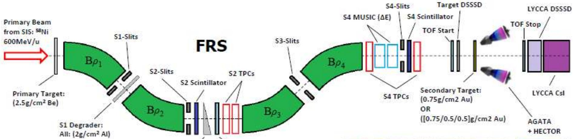
FRS ToF: S2 Sci  $\rightarrow$  S4 Sci ( $\beta\gamma$ )
