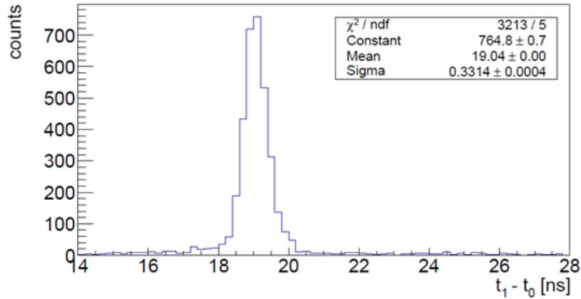
**Figure 5.5:** Time of flight measurement between Hodoscope ( $t_1$ ) and Start detector ( $t_2$ ) including the Cut1 correction. For more details see [6].
