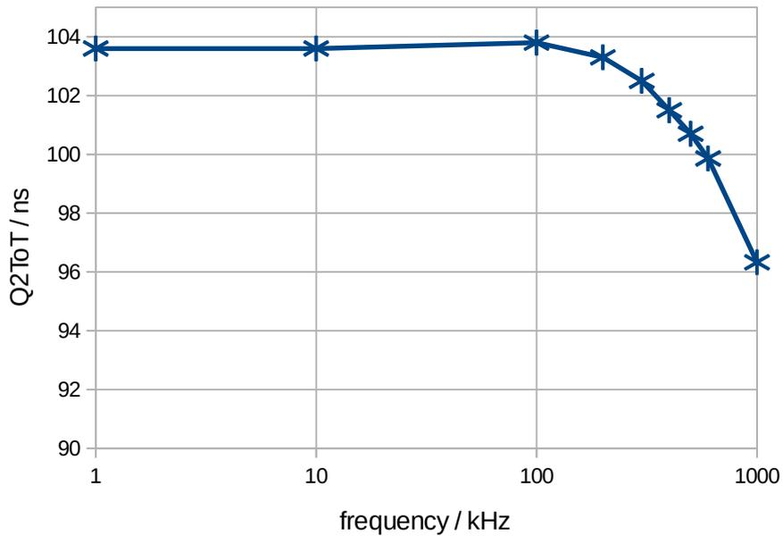
**Figure 3.10:** Rate capability for the first prototype. For rates above 100 kHz the measured Q2ToT decreases.
