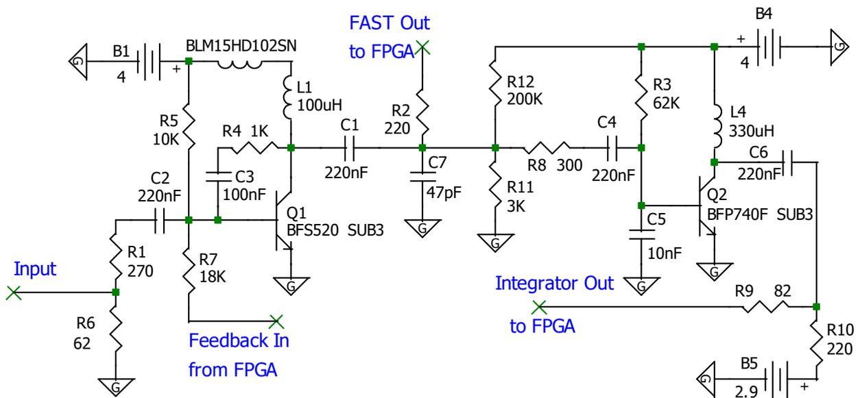
Figure 8.5: Current, optimized schematics of the analog part of PaDiWa-AMPS for Si-PM read-out.
