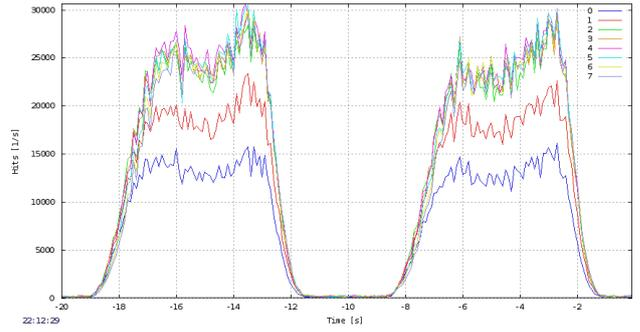
**Figure 5.3:** Examples of two quality assessment (QA) plots which have been displayed in the HADES control room during the pion beam time. **Left panel:** The hit rate per second is displayed for all PMTs of the Hodoscope. The y-profile of the beam is visible. **Right panel:** Hit rate of all eight rods as a function of time. The spill structure of the pion beam is visible.
