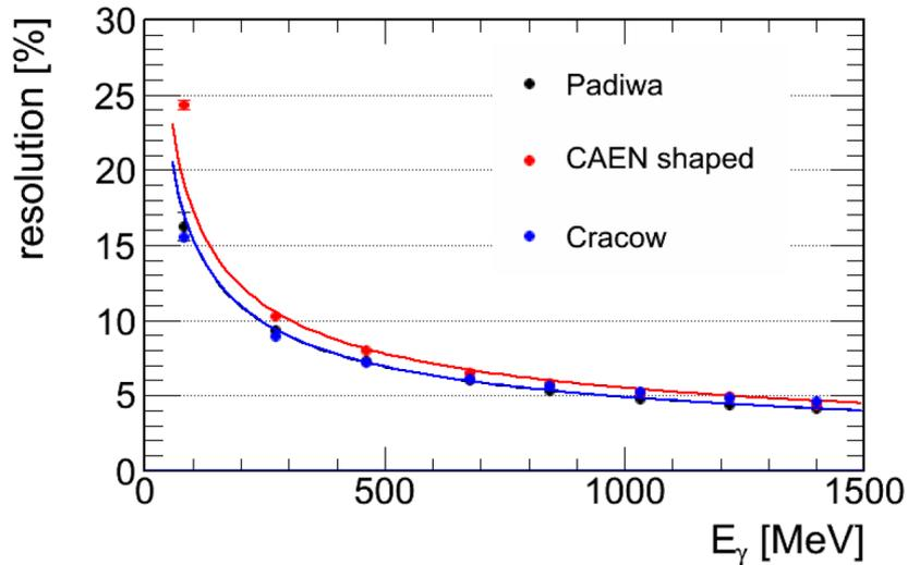
Figure 4.6: Comparison between all three tested read-out electronics for ECAL modules equipped with the 3 inch PMT types [50].
