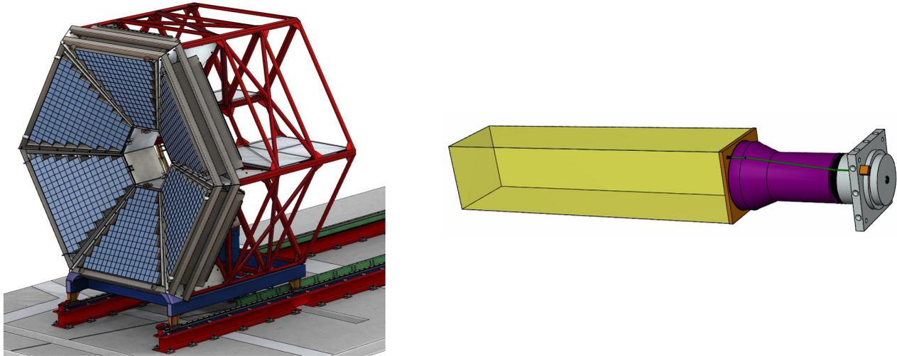
**Figure 1.14:** Left panel: 3D model of the HADES ECAL detector with about 1000 lead glass modules [25]. Right panel: Components inside an ECAL module consists of a lead glass block (yellow) coupled to a PMT (magenta). LED light for testing purposes can be inserted via an optical fiber (green). The lead glass is warped in Tyvek and a light tight brass box is used as housing (not shown) [14].
