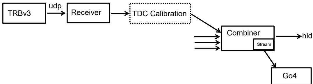
**Figure 2.7:** DABC and Go4 read-out scheme showing the data transport from the TRB3 board. An automatic TDC calibration can be performed in real time. It is also possible to calibrate the TDCs with calibration data generated from the hld file. This is useful for important data, because the automatic calibration can not be undone.
