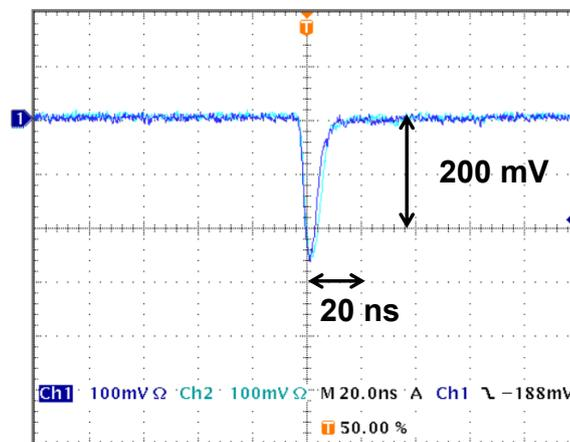
**Figure 5.1:** Hodoscope pulse shape generated by a cosmic muon. The plastic szintillators are read out from both sides using 0.5 inch Hamamatsu R3478 PMTs.
