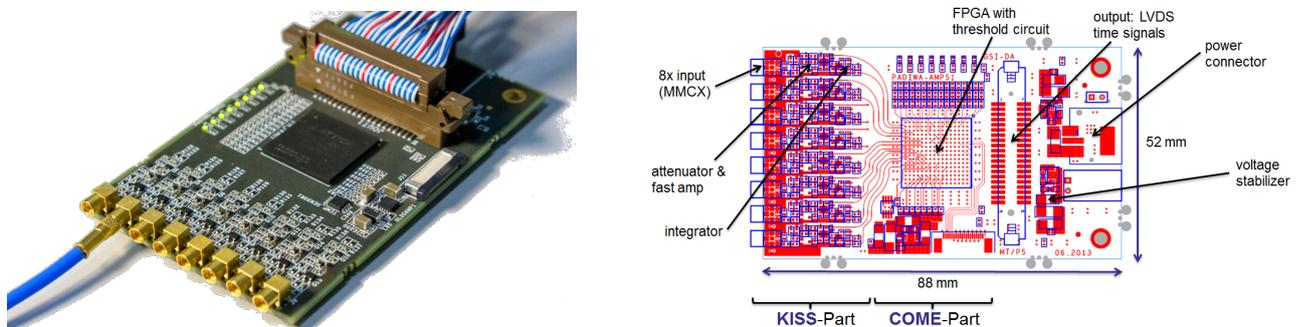
**Figure 2.5:** Left panel: Photograph of the first PaDiWa-AMPS front-end board prototype for the TRB3 platform. Right panel: Top view on the layout of PaDiWa-AMPS with some mayor parts marked. The full electronic schematics one can find in [42].
