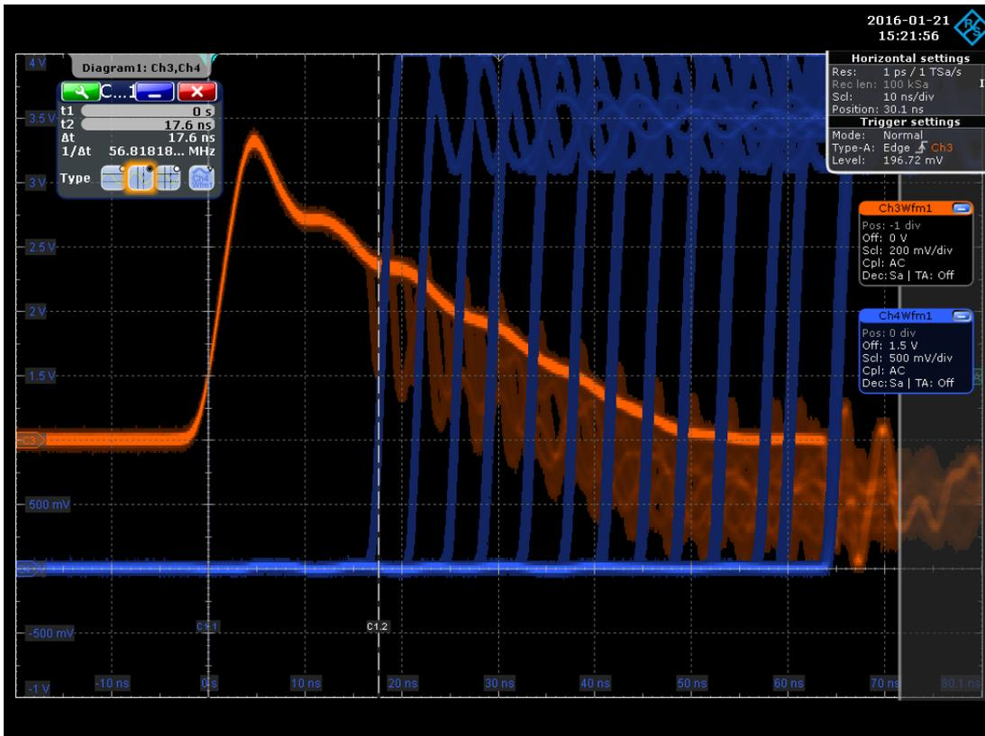
**Figure 6.18:** Selectable delays for the DISCHARGE signal are shown in blue. The FAST signal is shown in orange. Delays from 18 ns up to 65 ns can be selected in steps of about 4.5 n.
