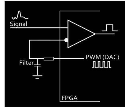
**Figure 2.1:** Left panel: Possible solution for a LVDS standard implementation with Lattice MachXO2 devices [35]. Right panel: Scheme of the signal discrimination via the LVDS input buffers. Thresholds to the input signals are set by an Digital-to-Analog-Converter (DAC) using Pulse Width Modulation (PWM) in combination with a low pass filter [36].
