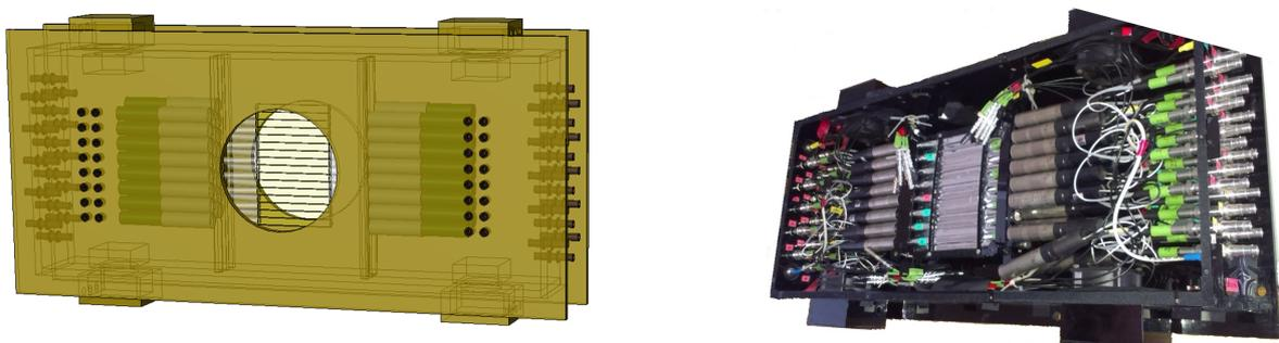
**Figure 1.6:** Schematic drawing (left panel) and photography (right panel) of the Hodoscope detector which belongs to the beam diagnostics system of the HADES. The Hodoscope consist of 16 horizontally aligned plastic scintillator rods. The scintillation light is read out at both ends by PMTs. The system is mounted in a light tight plastic housing [14].
