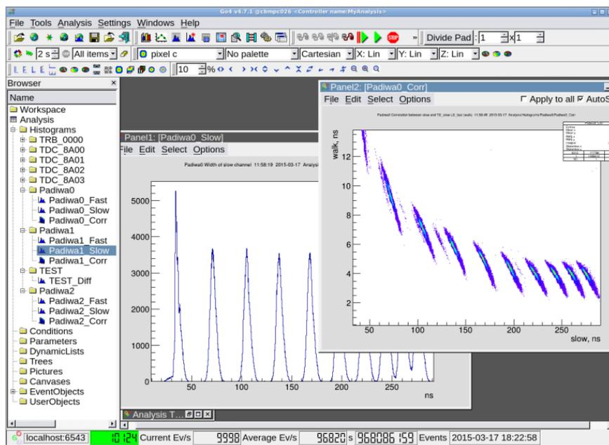
**Figure 2.8:** Screen-shot of the Go4 GUI. A ROOT based analysis can be displayed in real-time.
