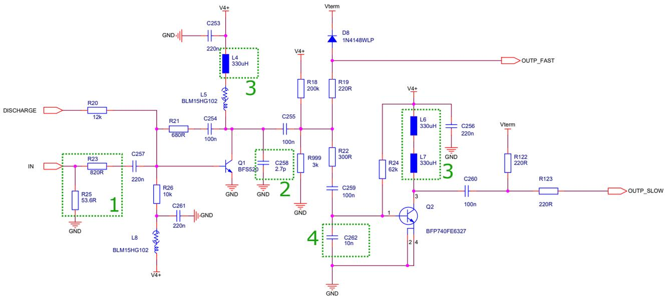
**Figure 2.4:** PaDiWa-AMPS electronics scheme for the first channel, excluding the FPGA. The elements which have been investigated to optimize the scheme to ECAL and other pulse shapes are labeled: 1) Attenuation part, 2) High frequency cut-off, 3) Low frequency cutt-off, 4) Integrator gain.
