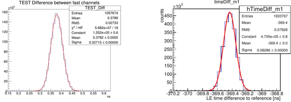
**Figure 3.6: Left panel:** Time difference between two channels by splitting the input signal. A time precision of  $\frac{\sigma_{t_1}}{\sqrt{2}} = 19$  ps was determined for a single channel. **Right panel:** Time difference relative to the trigger signal. A time precision of  $\sigma_{t_1 - t_{trigger}} = 83$  ps was determined.
