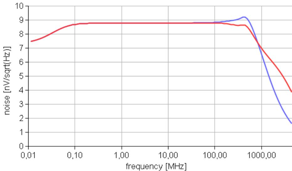
**Figure 6.8:** Frequency dependence of the normalized noise at the output of the FAST amplification stage for two values of the filter capacitor C258. Blue curve: 2.7 pF, Red curve: 1 pF.
