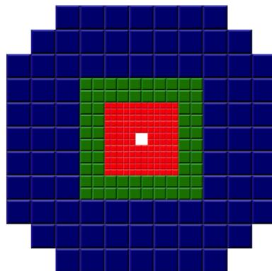
**Figure 1.13:** Schematic front view of the Forward Hodoscope Wall. The detector is made out of 228 plastic scintillation cells in three different dimensions which are indicated by the colors blue, green and red which are read out by PMTs [5].
