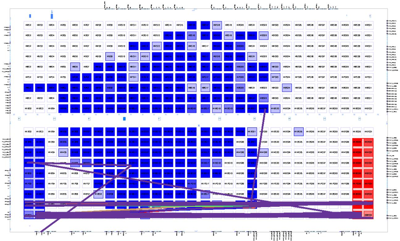
**Figure 6.16:** Floorplan view of the FPGA taken from the Lattice Diamond<sup>®</sup> Software. The stretchers are located in the left and right lower corners. The Magenta lines show the location of the instances which are needed to generate and delay the DISCHARGE signal.
