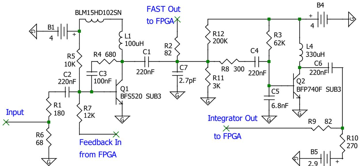
Figure 8.4: Current, optimized schematics of the analog part of PaDiWa-AMPS for HADES Hodoscope and Diamond Detector read-out.
