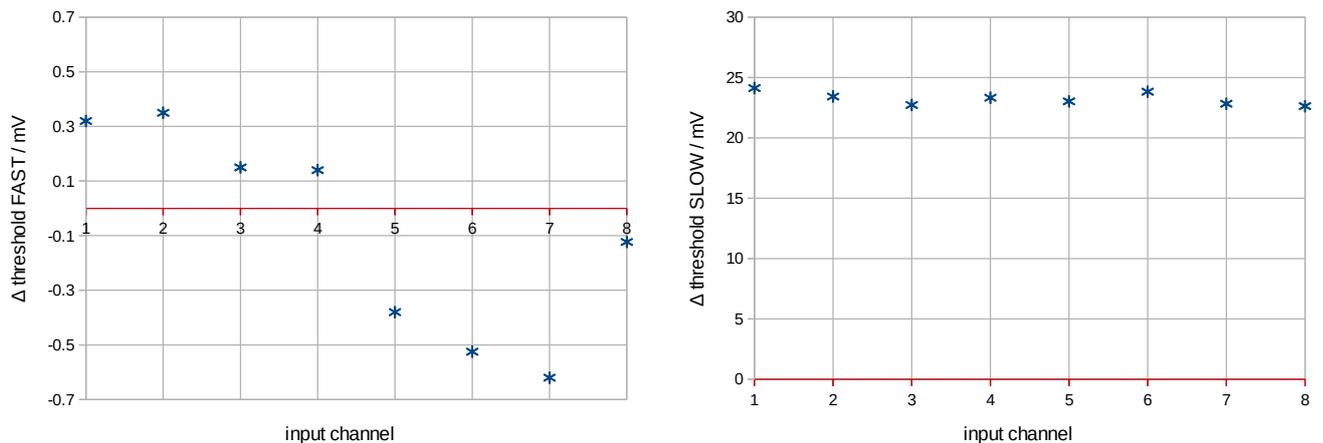
**Figure 3.3:** Deviations of measured threshold voltages on the board for a fixed set threshold in the PaDiWa-AMPS control GUI. The FAST channels (left panel) were set to 100 mV. The maximum deviation is about 0.6 mV. The SLOW channels (right panel) were set to 2850.3 mV. An offset of about 25 mV is observed, but the deviation around the offset is below 2 mV.
