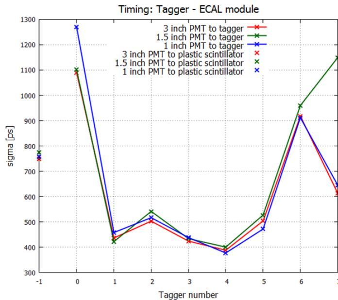
**Figure 4.9:** Time precision between the additional plastic scintillator and ECAL module (Tagger number -1) and between the eight Tagger channels and the ECAL module (Tagger number 0-7). The strong variation of the time precision indicates that the precision is dominated by the Tagger electronics.
