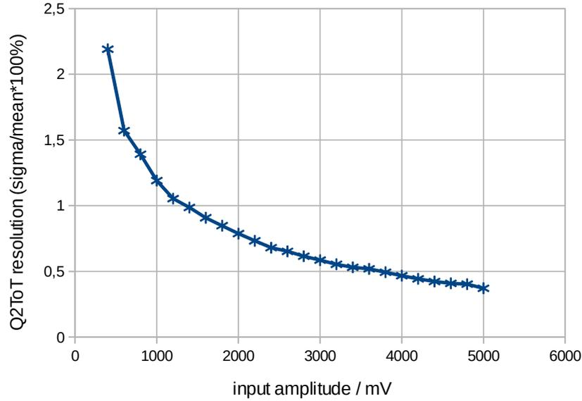
**Figure 3.7:** Relative charge resolution, which is defined by  $\sigma/\text{mean} \cdot 100$  [%], for different input amplitudes. Signals with variable amplitude from a laboratory pulses with similar shape as HADES ECAL pulses have been used. For signals amplitudes above 1.5 V the resolution is below 1%.
