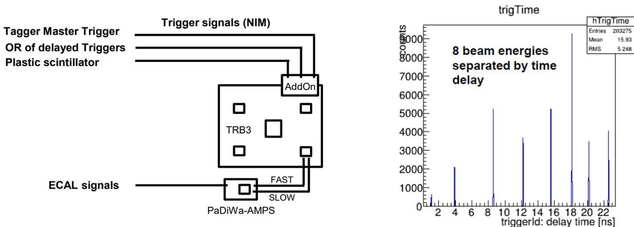
**Figure 4.3:** Left panel: Schematic picture of the PaDiWa-AMPS readout scheme. The ECAL modules were connected to the PaDiWa-AMPS front-end board which is connected to the TRB3. Master Trigger, delayed trigger OR and discriminated signal of the additional plastic scintillator were connected to a GPin AddOn board. Right panel: The eight gamma energies were separated by generating a logical OR with the different delays (right panel).
