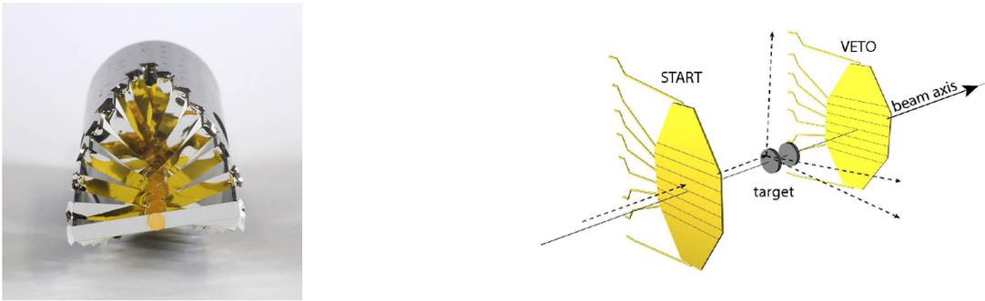
**Figure 1.4:** Left panel: Photography of the Gold target which was used in the HADES Au+Au beam time in 2012. It is segmented into 15 segments, with a thickness of  $25\ \mu\text{m}$ , which are mounted in a carbon fiber support. (Picture by Gabi Otto, GSI) Right panel: Schematic view of the Start-Target-Veto System as it was used in the same Au+Au beam time [5].
