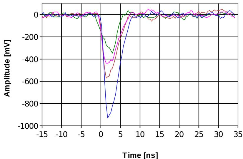
**Figure 6.3:** Pulse shapes from  $500\ \mu\text{m}$  thick mono crystalline diamond detector which is irradiated with a Sr-90 source (equivalent to MIPS), measured after pre-amplifier & booster/shaper amplifier.
