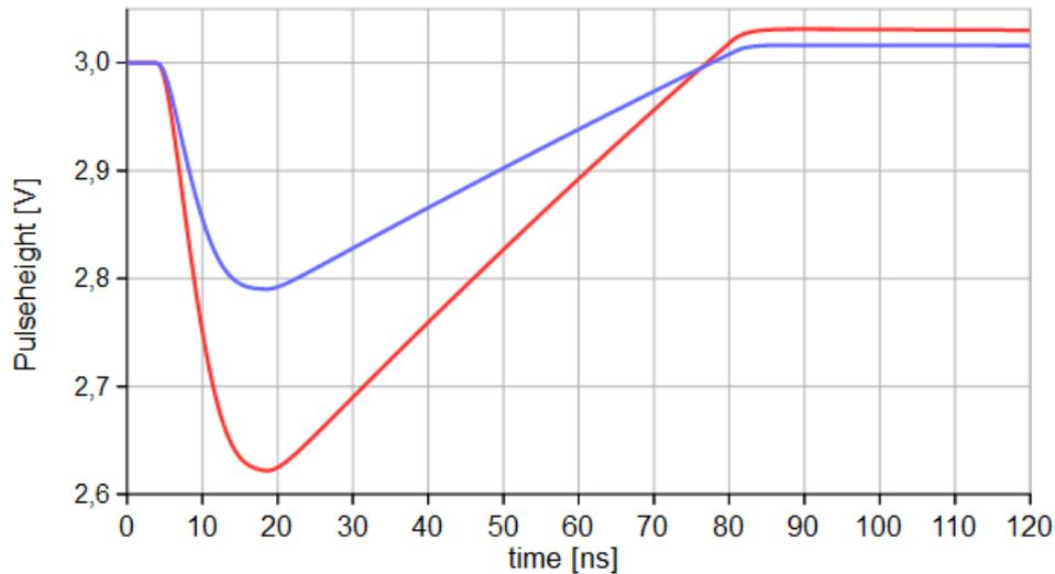
**Figure 6.11:** Simulated SLOW output for a typical Hodoscope or Diamond Detector signal with an amplitude of 0.5 V. The result for the standard ECAL version is shown with the blue. The integrating capacitor is decreased from 10 nF to 6.8 nF and the termination resistor is increased from  $220\ \Omega$  to  $270\ \Omega$ . The resulting signal with the red curve shows the higher gain of the integrator.
