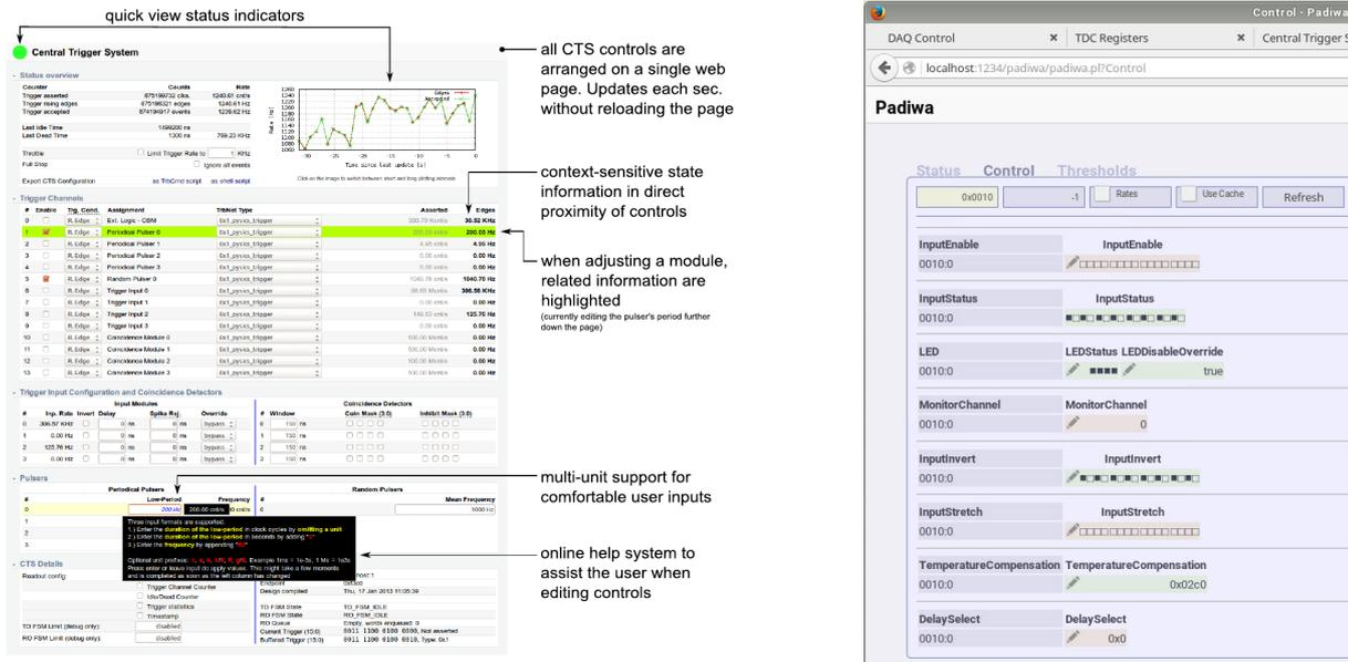
**Figure 8.2:** Left panel: Screen-shot of the HTML based CTS GUI. It shows the main page of the Central Trigger System [10]. Right panel: Screen-shot of the PaDiWa-AMPS slow control main page. Input channels can be enabled and the delay of the discharge signal can be set.
