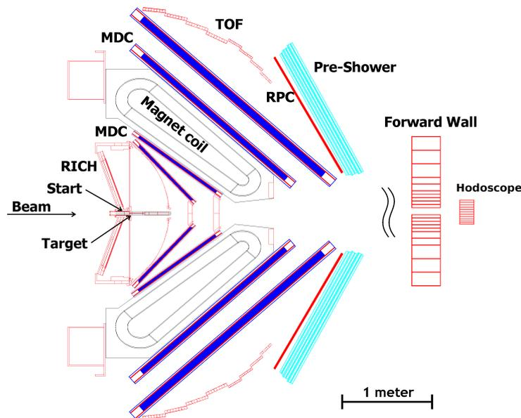
**Figure 1.3:** Transverse section view of the HADES detector layout as it was used during the pion beam experiments in Summer 2014. As already mentioned the Pre-Shower detector will be replaced in future by an Electromagnetic Calorimeter (ECAL) [6].
