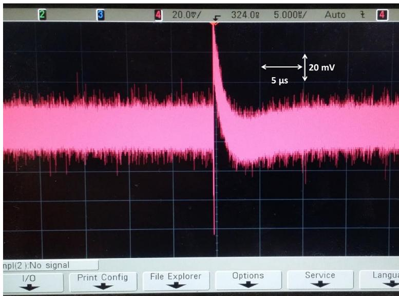
**Figure 3.11:** The rate capability is limited by an overshoot in the SLOW signal which has a natural decay time in the order several  $\mu$ s.
