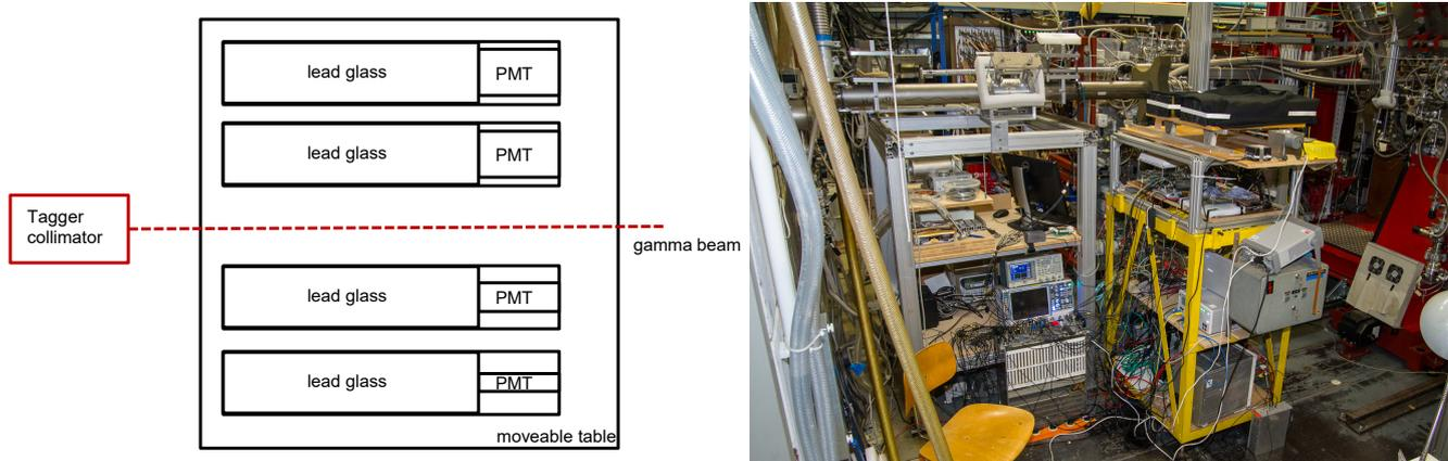
**Figure 4.2:** Left panel: Schematic top view of the movable platform, equipped with four ECAL modules. The front plate of the modules were located 1 m downstream of the tagger exit window (marked as a red box). Right panel: Photography of the ECAL test set-up. The movable table equipped with the ECAL modules is placed on a yellow support frame. Beam direction is from left to the right side. Trigger and read-out electronics are placed under the movable platform and in a second shelf.
