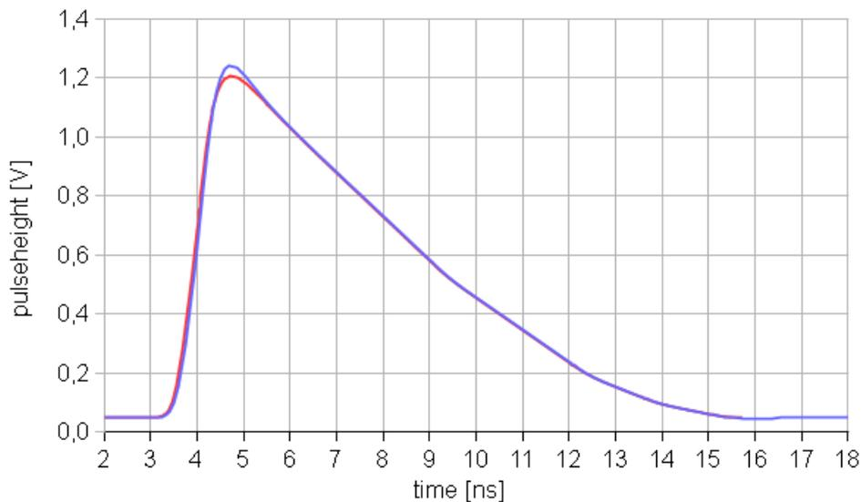
**Figure 6.9:** Amplified FAST signal for two values of the filtering capacitor C258. Blue curve: 2.7 pF, Red curve: 1 pF. The total rise-time of the input signal is 1 ns what is comparable to a Diamond or a fast Hodoscope PMT signal.
