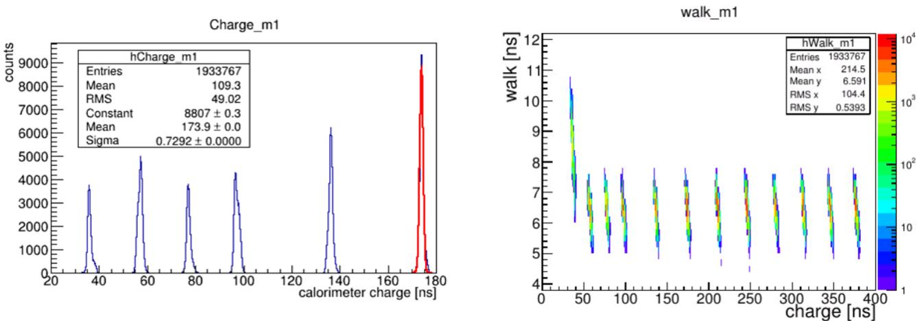
**Figure 3.8: Left panel:** Typical result from a charge measurement. The amplitude of the input pulse was varied while holding the width of the pulse constant. Here the width of the SLOW signal is defined by trailing edge of SLOW minus leading edge of FAST. After fitting with a Gaussian the mean and sigma is used for the characterization. **Right panel:** Walk effect which can be corrected offline to improve the charge resolution especially for small signal amplitudes.
