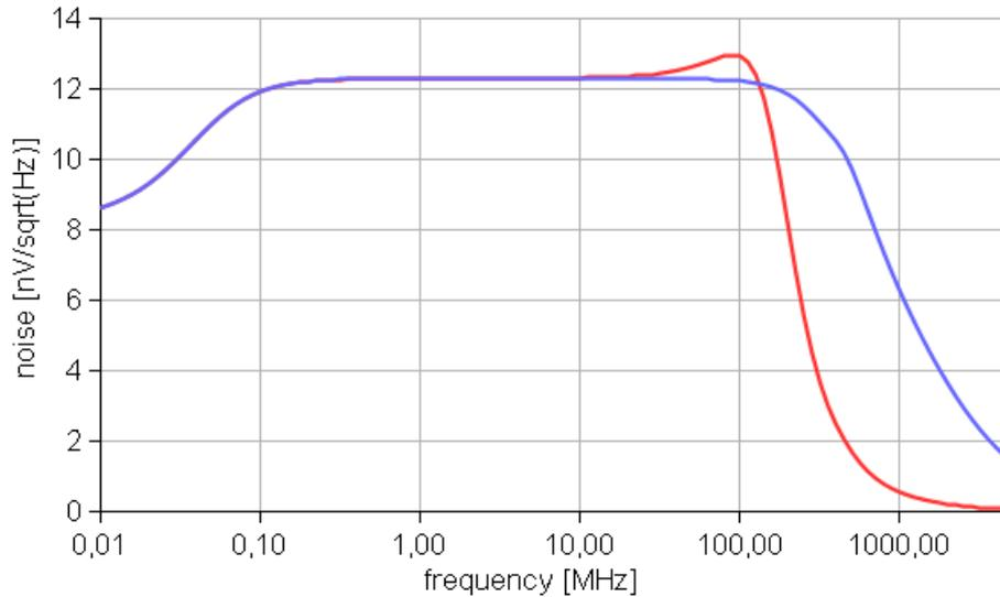
**Figure 6.6:** Frequency dependence of the normalized noise at the output of the FAST amplification stage for two values of the filter capacitor C258. Blue curve: 2.7 pF, Red curve: 47 pF.
