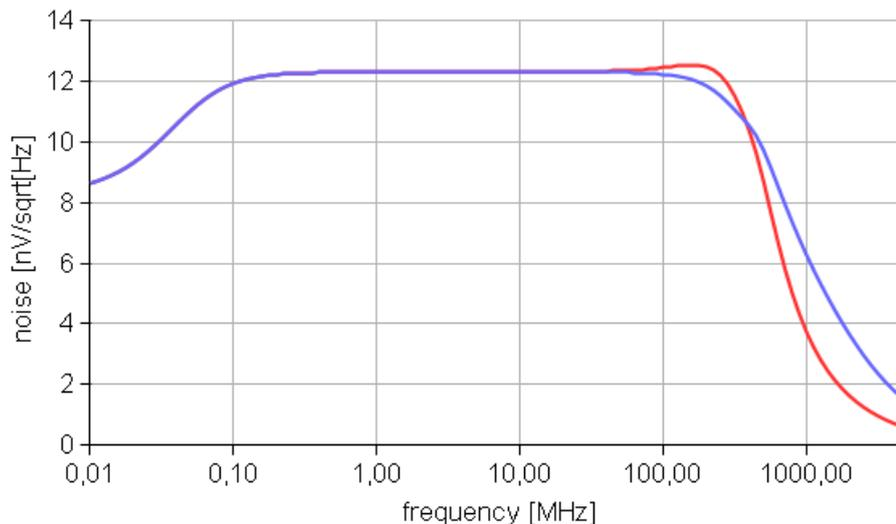
**Figure 6.4:** Frequency dependence of the normalized noise at the output of the FAST amplification stage for two values of the filter capacitor C258. Blue curve: 2.7 pF, Red curve 6.8 pF.
