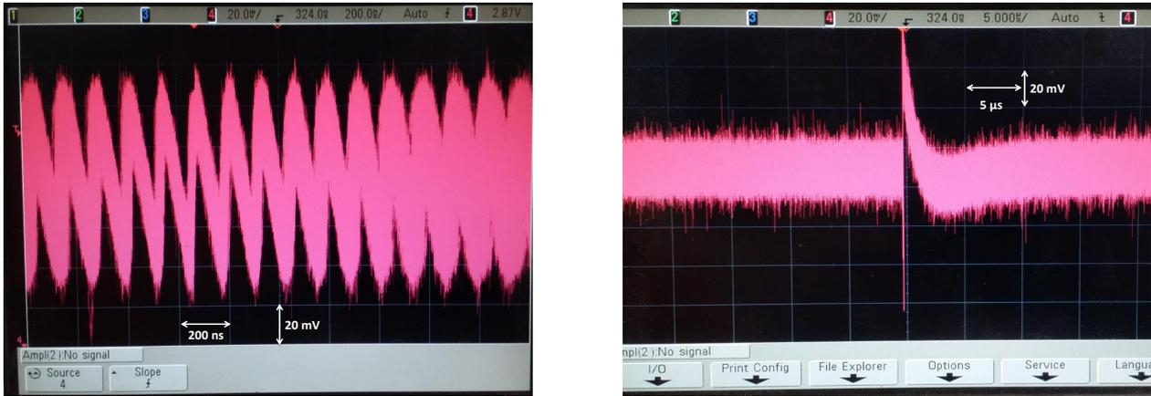
**Figure 6.15:** Left panel: Oscillation in the SLOW signals which starts for very low relative threshold values. The oscillation is caused by re-triggering on an undershoot which is related to the overshoot in the SLOW signal. Right panel: The undershoot is especially visible for small input signals. To avoid the re-triggering, the DISCHARGE signal must require the FAST signal which is not affected by re-triggering.
