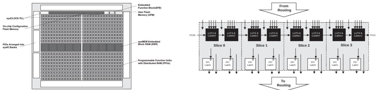
**Figure 8.1:** Left panel: Top-level architecture block diagram of the LATTICE MachXO2-400HC PLD [35]. Right panel: A Programmable Functional Unit (PFU) block consists out of four interconnected slices. Each slice contains two LUTs and two registers (Flip-Flop or Latch). There are 53 inputs and 25 outputs associated with each PFU block [35].
