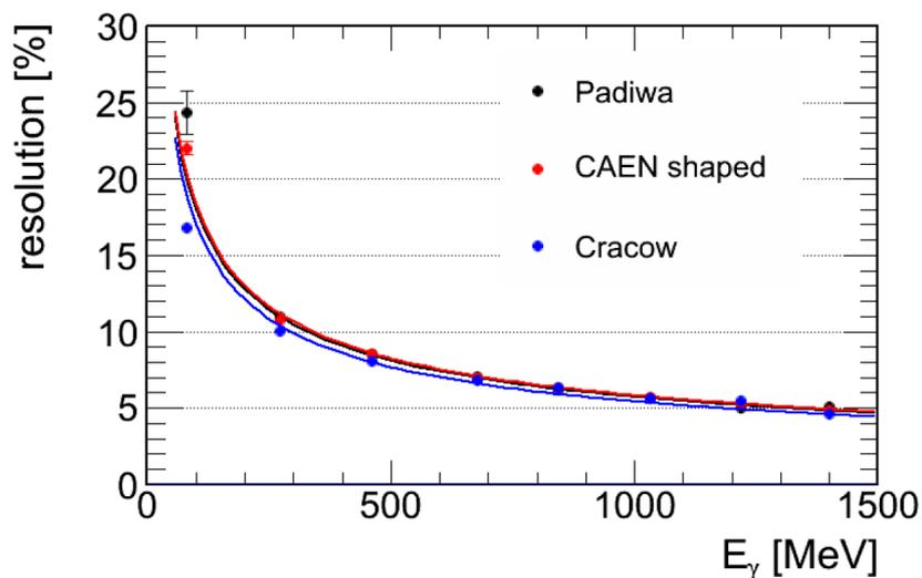
Figure 4.7: Comparison between all three tested read-out electronics for ECAL modules equipped with the 1.5 inch PMT types [50].
