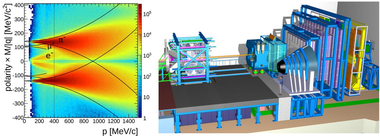
**Figure 1.2: Left panel:**  $M/|q|$  times polarity as a function of particle momentum  $p$  reconstructed with the RPC detector. Electron/pion separation at large momenta can be improved by including an electromagnetic calorimeter (ECAL) into the HADES set-up. **Right panel:** Artist view of the experimental cave housing the HADES and the CBM experiment at the future FAIR accelerator complex [5].
