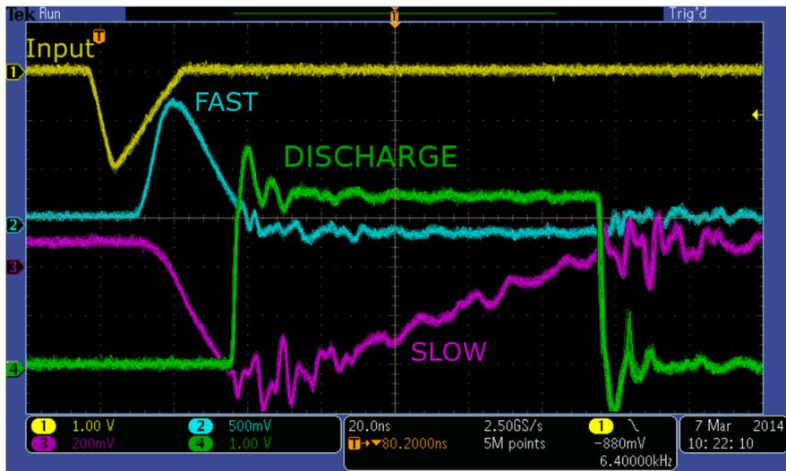
**Figure 3.2:** Scope picture showing some characteristic analog signals, probed on the PaDiWa-AMPS board. The yellow signal shows the input signal which was generated by a pulser. The blue signal shows the FAST signal (measured over R19). The DISCHARGE signal (measured over R20) is shown in green. The SLOW signal (measured over R123) is shown in magenta. Signal reflections are mainly introduced by the probe. Taken from [49].
