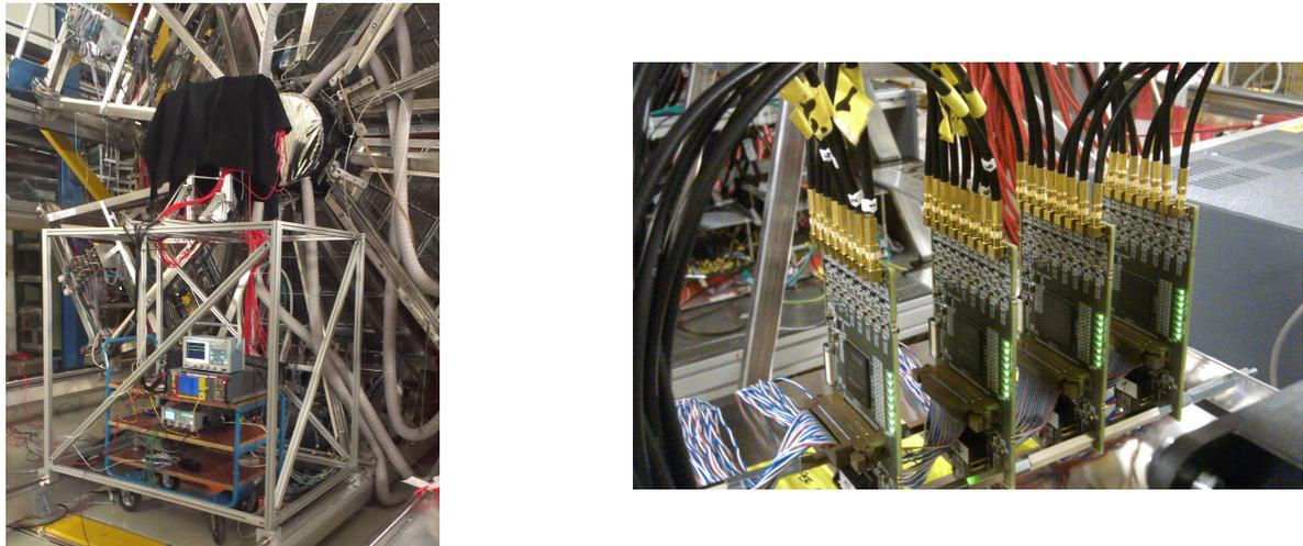
**Figure 5.2:** **Left panel:** Hodoscope detector set-up seen from the back side of the HADES. The movable platform contains the Hodoscope (covered with a black blanket), HV-Supply and read-out electronics. **Right panel:** Four modified PaDiWa-AMPS boards in combination with a TRB3 have been used to read out the 32 channels of the Hodoscope detector.
