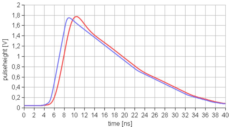
**Figure 6.7:** Amplified FAST signal for two values of the filtering capacitor C258. Blue curve: 2.7 pF, Red curve: 47 pF. The total rise-time of the input signal is 5 ns which is comparable to PSD Si-PM signals.
