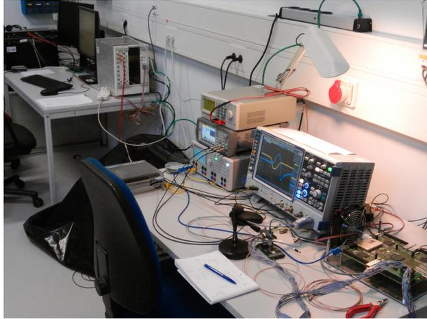
**Figure 3.1:** Set-up for the characterization of the PaDiWa-AMPS prototype board, located in the Detector Laboratory (DL) of GSI. The PaDiWa-AMPS board is connected to a TRB3, which is connected to personal computer via Ethernet. Test signals generated by laboratory pulse generators and ECAL modules can be used to test the performance of front-end board.
