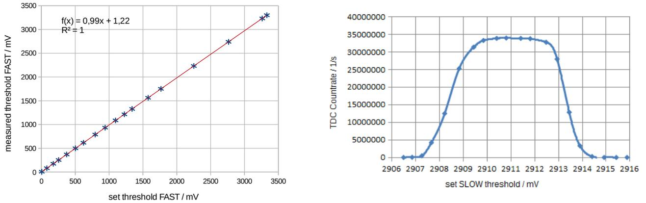
**Figure 3.4:** **Left panel:** The measured threshold on the board shows a linear behavior with a small offset to the threshold set in the GUI. **Right panel:** The TDC count rate (obtained from the CTS GUI) as a function of the set threshold for a SLOW channel. The flat top of the distribution is due to the FPGA-TDC counting rate limitation of the TRB3 board.
