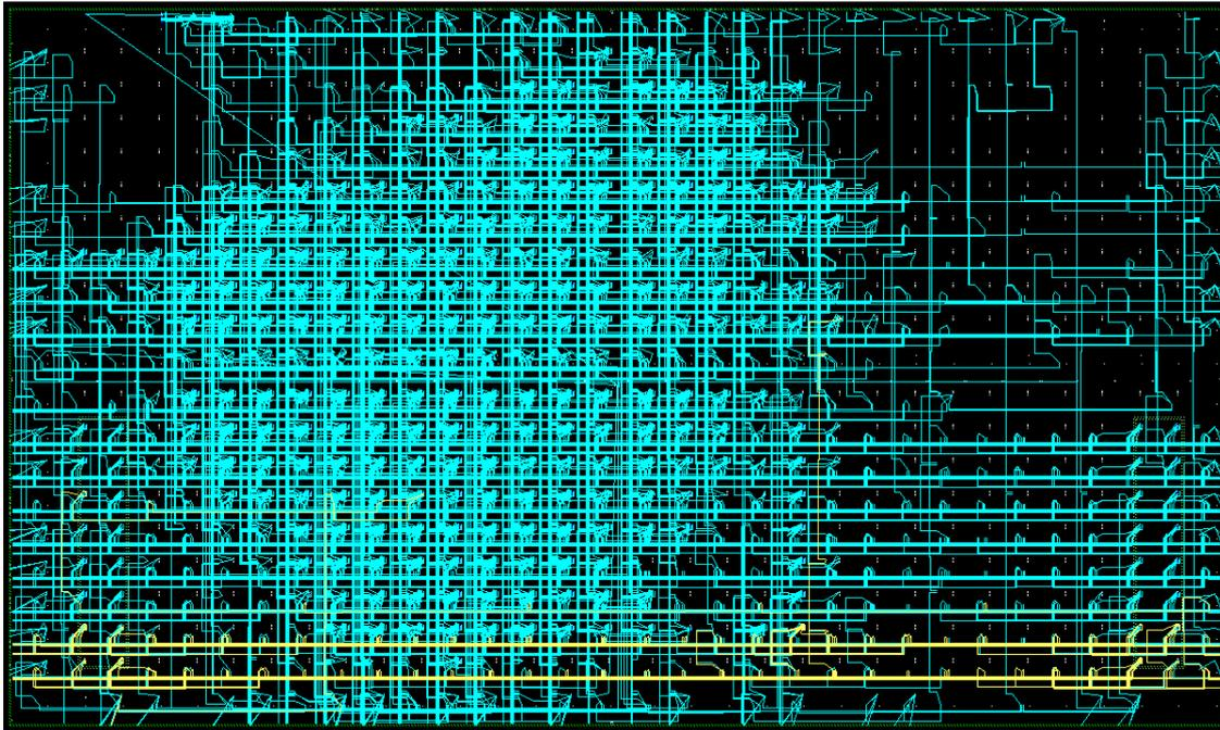
**Figure 6.17:** Physical view taken from the Lattice Diamond® Software. All paths inside the FPGA are shown in blue. The signal line of the DISCHARGE signal is shown in yellow. Starting at the FAST input, to the place where the DISCHARGE signal is generated. From there it is routed through the Stretcher and ends at the Multiplexer, which allows the selection of the delay. From the Multiplexer it is routed to the output pad.
