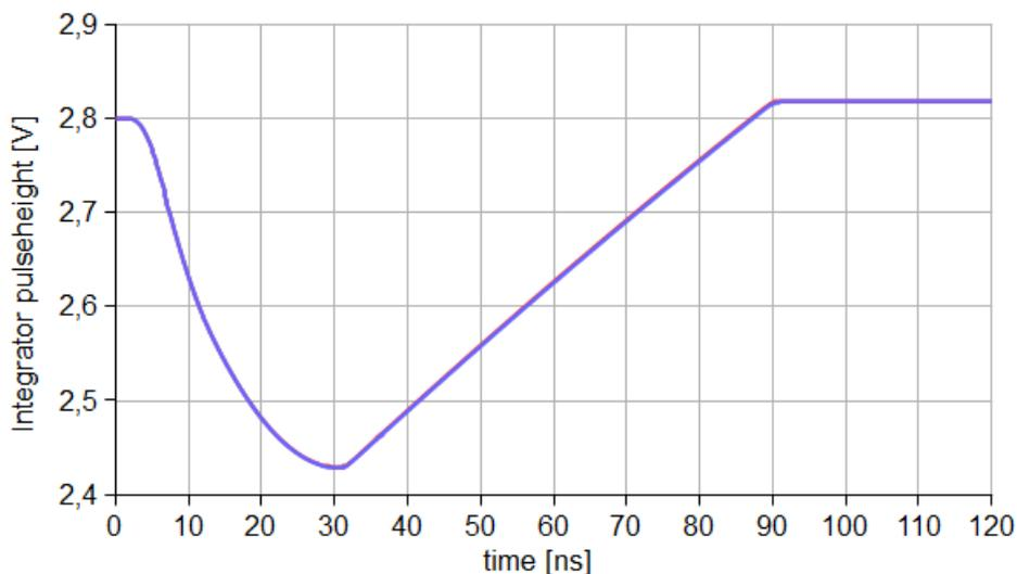
**Figure 6.13:** Integrated SLOW output signal simulated for an ECAL PMT shaped input signal with an amplitude of 0.7 V for two different values of the blocking inductor  $L_4$ . Blue curve:  $330 \mu\text{H}$ , Red curve:  $100 \mu\text{H}$ . Blue curve and red curve fall on top of each other.
