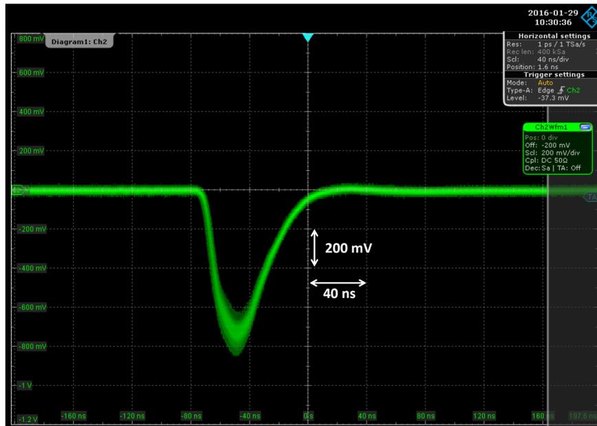
**Figure 6.1:** Si-PM pulse generated by a Hamamatsu S12572 MPPC which was irradiated with short LED pulses.
