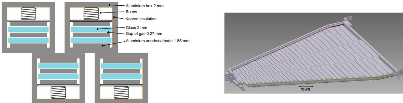
**Figure 1.11:** Left panel: The HADES multi-gap RPC cell layout and their ingredients. The cells are aligned in two overlapping rows [22]. Right panel: A schematic drawing of a RPC sector. The cells have smaller sizes at smaller polar angles and fill the trapezoidal support frame [5].
