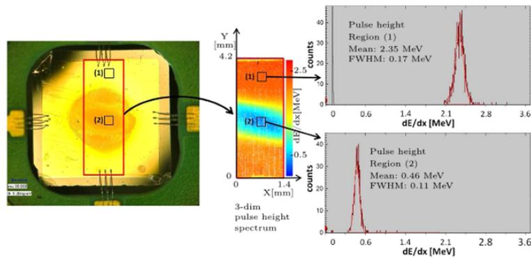
**Figure 6.2:** Left panel: HADES Diamond detector after irradiation with Gold ions. Middle panel: The distribution of energy loss of pulse height spectrum. Right panel: Pulse height for two regions on the diamond. Top panel: less irradiated area, bottom panel highly irradiated area [8].
