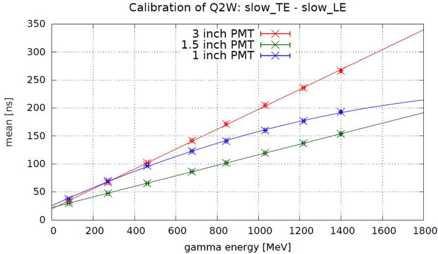
**Figure 4.4:** The calibration curves for 3 and 1.5 inch PMT modules show a linear behavior. The module equipped with a 1 inch shows a saturation effect, caused by the high voltage which was close to the maximum operating voltage recommended by the manufacturer. By fitting a linear and polynomial function respectively the relative energy resolution could be calibrated.
