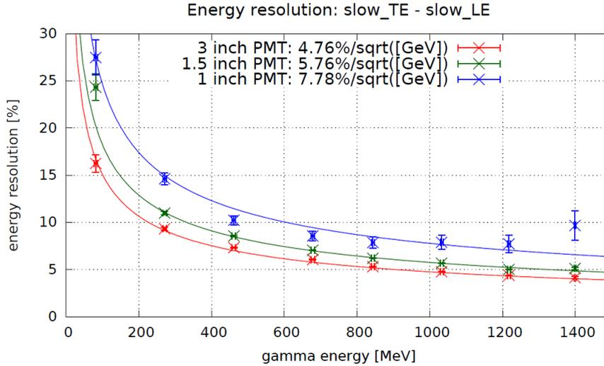
**Figure 4.5:** Calibrated relative energy resolution for all three PMT types.
