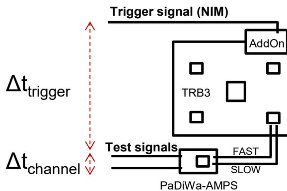
**Figure 3.5:** Laboratory set-up for the characterization of the time resolution.
