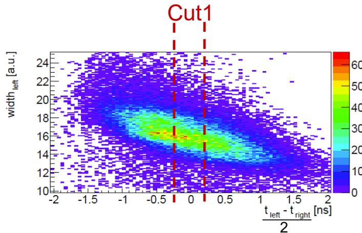
**Figure 5.4:** Walk effect of the position measurement along a Hodoscope rod. The time difference between left and right read out PMT as a function of the SLOW signal width (Q2ToT) is shown. **Right panel:** Time of flight measurement between Hodoscope and Start detector without corrections. For more details see [6].
