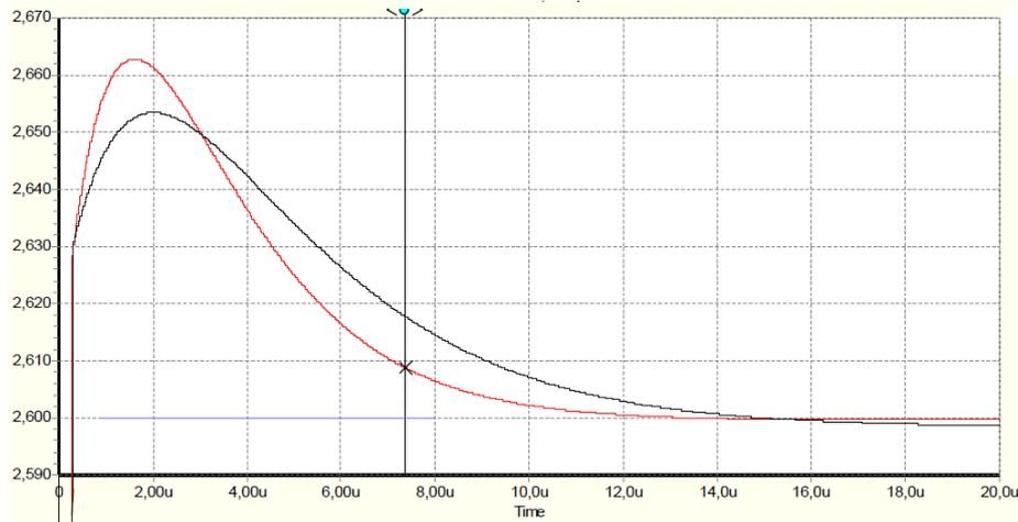
**Figure 6.14:** The decay time of the overshoot can be reduced by replacing the  $660 \mu\text{H}$  (black) blocking inductance (L6 + L7, see 2.4) by  $300 \mu\text{H}$  (red). This allows a higher rate capability.
