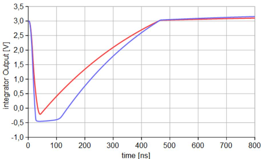
**Figure 6.10:** Simulated SLOW output for a typical PSD Si-PM signal with an amplitude of 2 V. The result for the standard ECAL version is shown with the blue curve. The integrating capacitor is increased from 10 nF to 12 nF and the termination resistor is reduced from 220  $\Omega$  to 200  $\Omega$ . The resulting signal shown with the red curve does not indicate saturation.
