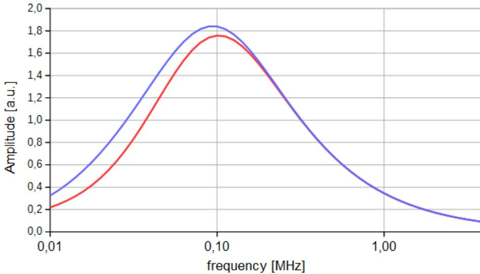
**Figure 6.12:** Frequency dependence of the gain of the SLOW integrator for two different values of the blocking inductor  $L_4$ . Blue curve:  $L_4 = 330 \mu\text{H}$ , Red curve:  $L_4 = 100 \mu\text{H}$ . A gain reduction of about 50% in the low frequency range of a few 10 kHz is visible.
