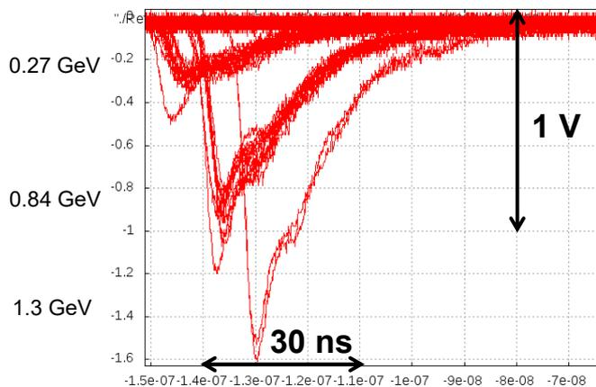
**Figure 1.15:** Typical pulse shapes from an ECAL module, recorded with an oscilloscope. The module was equipped with a 3 inch HAMAMATSU R6091 PMT and irradiated with three different gamma energies. Important for the adaption of the read-out electronics is the rise-time (about 2.5 ns), the fall-time (about 40 ns) and the dynamic range of the amplitude.
