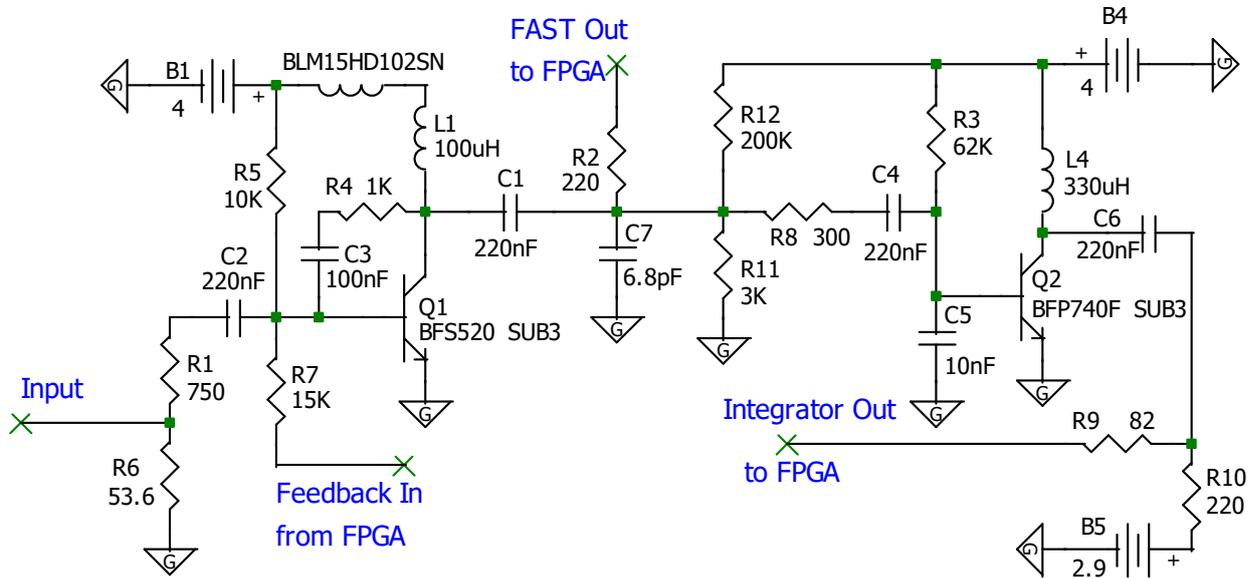
Figure 8.3: Current, optimized schematics of the analog part of PaDiWa-AMPS for HADES ECAL read-out.
