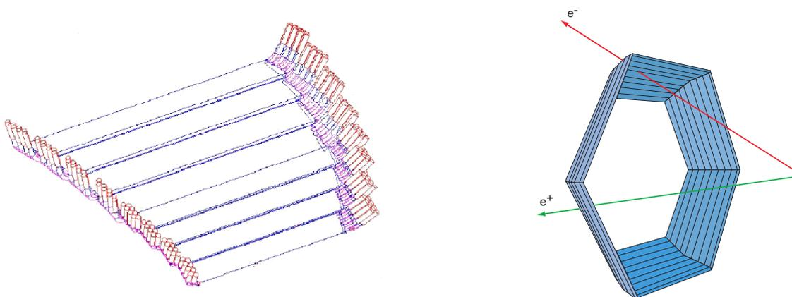
**Figure 1.10:** Left panel: Schematic layout of one sector of the Time of Flight Wall consisting of eight boxes of plastic scintillator stripes. The strip width is decreasing at lower polar angles to deal with the higher particle flux. Scintillation light is guided to the ends of the stripes where light guiders transport the light to the PMTs [5]. Right panel: Layout of the TOF detector showing the detection of an electron and a positron in two different sectors [5].
