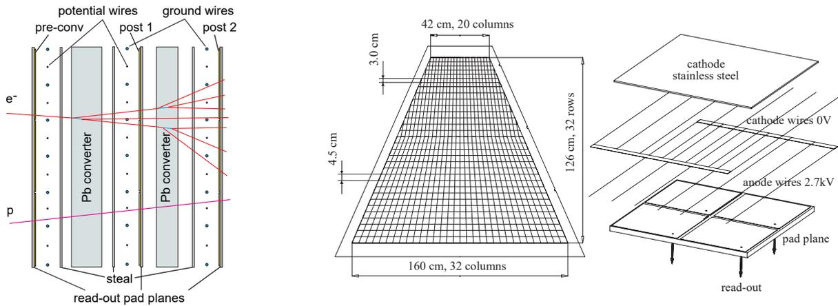
**Figure 1.12:** Left panel: Schematic side view drawing of the Pre-Shower Detector. An electromagnetic shower produced by an electron is much more pronounced than a hadronic shower induced by a proton [1]. Right panel: Schematic drawing of a wire chamber which is used to detect the shower which are created in the lead material [1].
