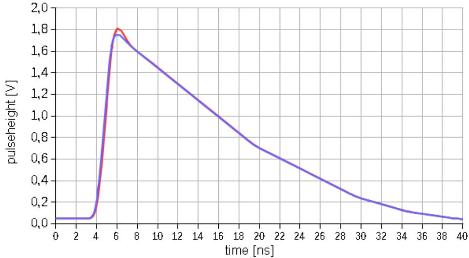
**Figure 6.5:** Amplified FAST signal for two values of the filtering capacitor C258. Blue curve: 2.7 pF, Red curve: 6.8 pF. The total rise-time of the input signal is 2 ns which is comparable to ECAL PMTs.
