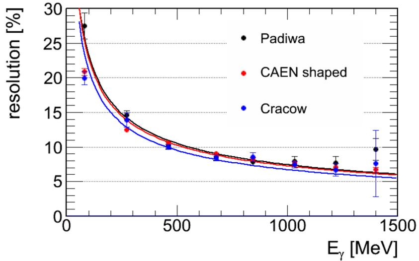
**Figure 4.8:** Comparison between all three tested read-out electronics for ECAL modules equipped with the 1 inch PMT types [50].
