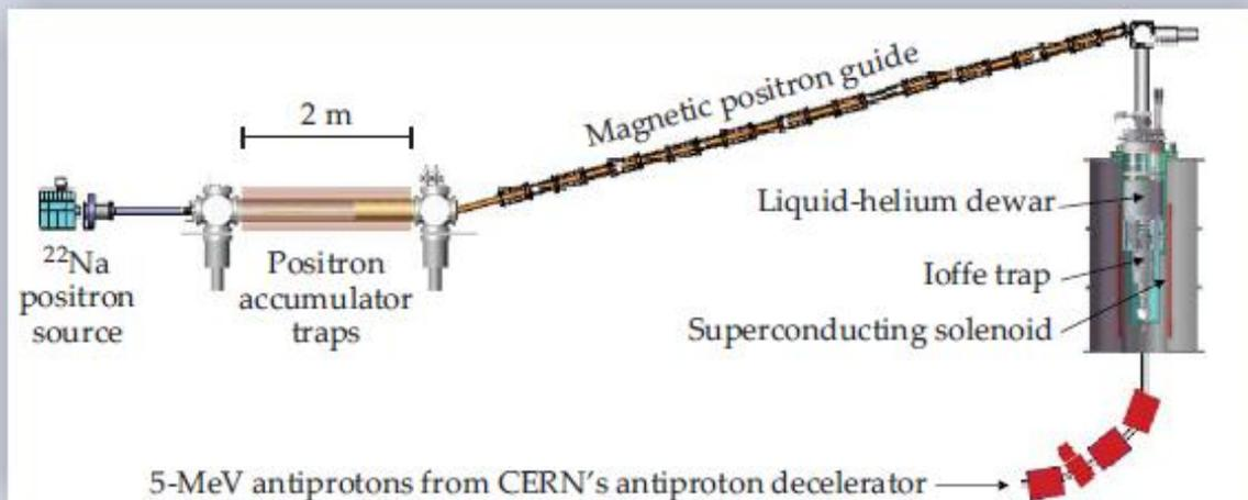
**Figure 1.** Key components of the ATRAP apparatus that accepts antiprotons from the antiproton decelerator at CERN and slows positrons from a sodium-22 source. The goal of the experiment is to trap and study cold antihydrogen atoms in the specially designed magnetic fields of the Ioffe trap.
