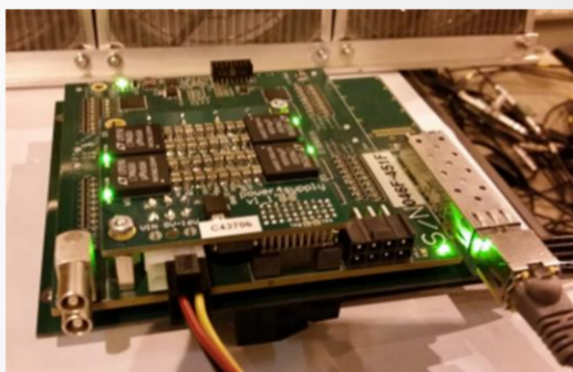
BM@N Readout electronics: FPGA based 64 channel ADC64 board, 62.5MS/s (AFI Electronics, JINR, Dubna).
