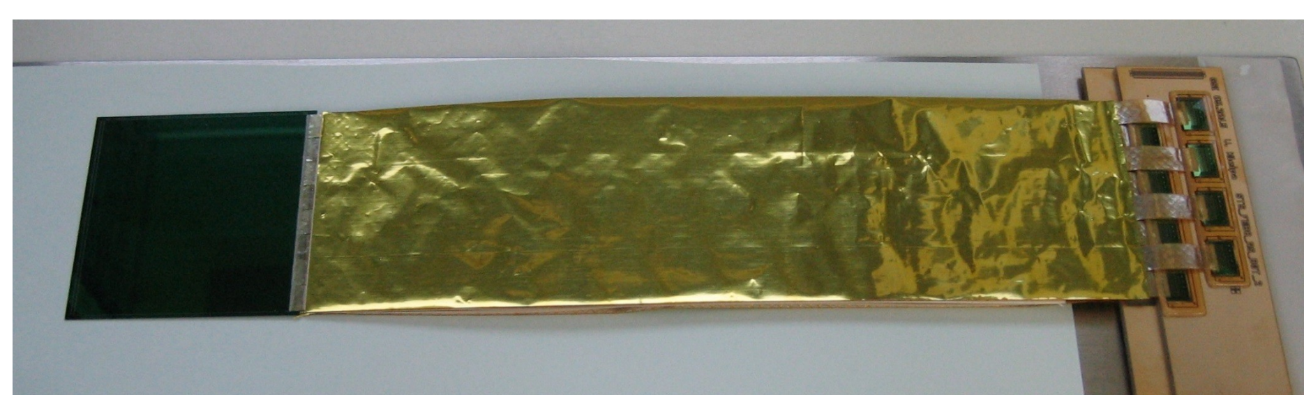
STS-module consists of a double-sided silicon microstrip sensor connected via microcables to two front-end-electronics PCB's
