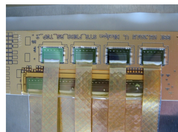
Die and wire-bonding of ASICs to the first row of FEB-8, after quality measurement procedure is repeated for second row
