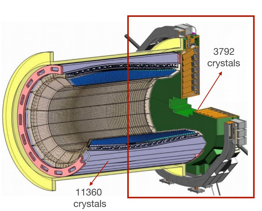
In total: 15744 lead tungstate crystals
