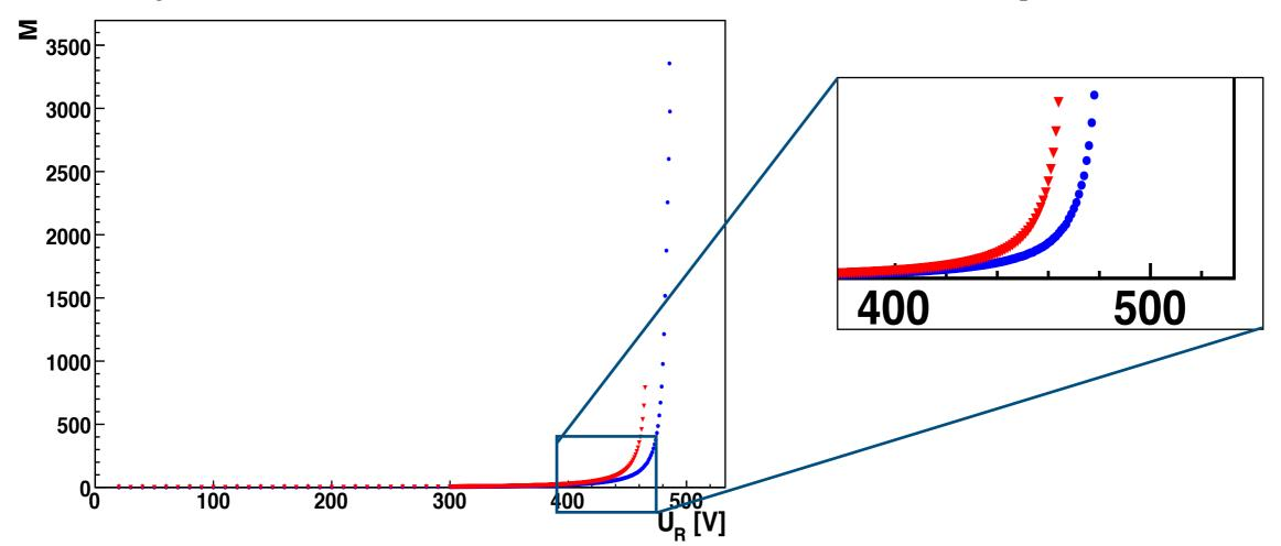
Radiation exposure causes shift in the high voltages of ~20 V for M=200.
