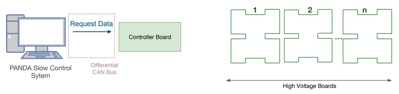
The PANDA Slow Control system issues readout request via Can Bus.
