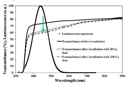
The irradiation leads to the population of color centers (induced absorbtion) => Degragation of the transmission
