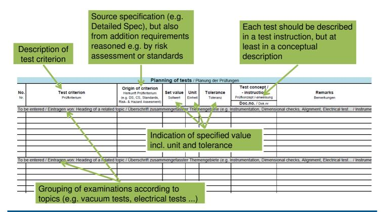
The part "Result / Ergebnis" can be used as cover sheet for the acceptance tests
