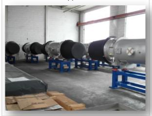
SIS100 quadrupole units shipped from JINR to BNG for integration in FOS module
