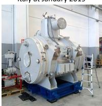
Copper plating and first tests of the RFQ accelerator cavity for the pLinac have been completed and match specifications
