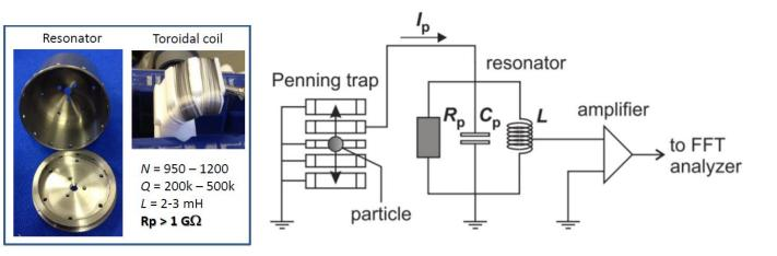
How do we measure the frequencies  $v_z$ ,  $v_+$  and  $v_-$ ?
