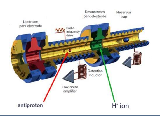
$$R = \frac{v_{c,\overline{p}}}{v_{c,H^-}} = \frac{(q/m)_{\overline{p}}}{(q/m)_{H^-}} \times \frac{B/2\pi}{B/2\pi}$$
