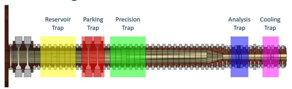
**Precision Trap**: Homogeneous field for frequency measurements, B2< 0.5 mT / mm2.
