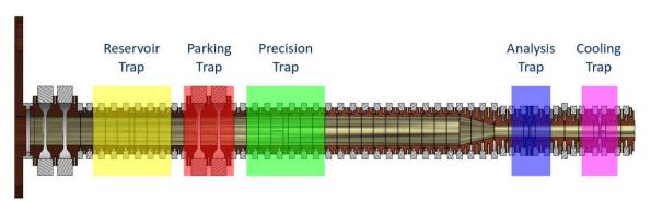
**Precision Trap**: Homogeneous field for frequency measurements, B2< 0.5 mT / mm2.
