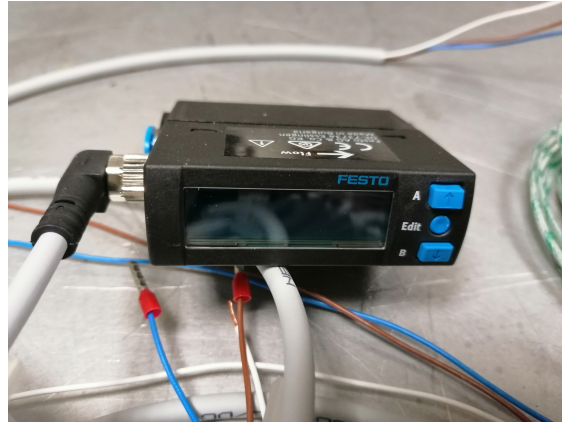
Flow meter (FESTO) from 0.002 l/min to 200 l/min
