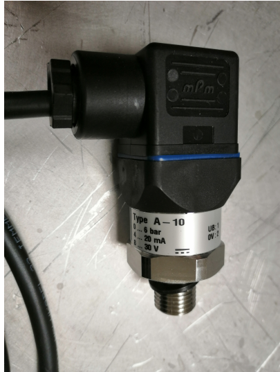
Pressure sensor (Wika) A-10, 0 – 1000 bar
