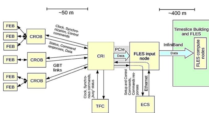
Block diagram of the STS Readout chain
