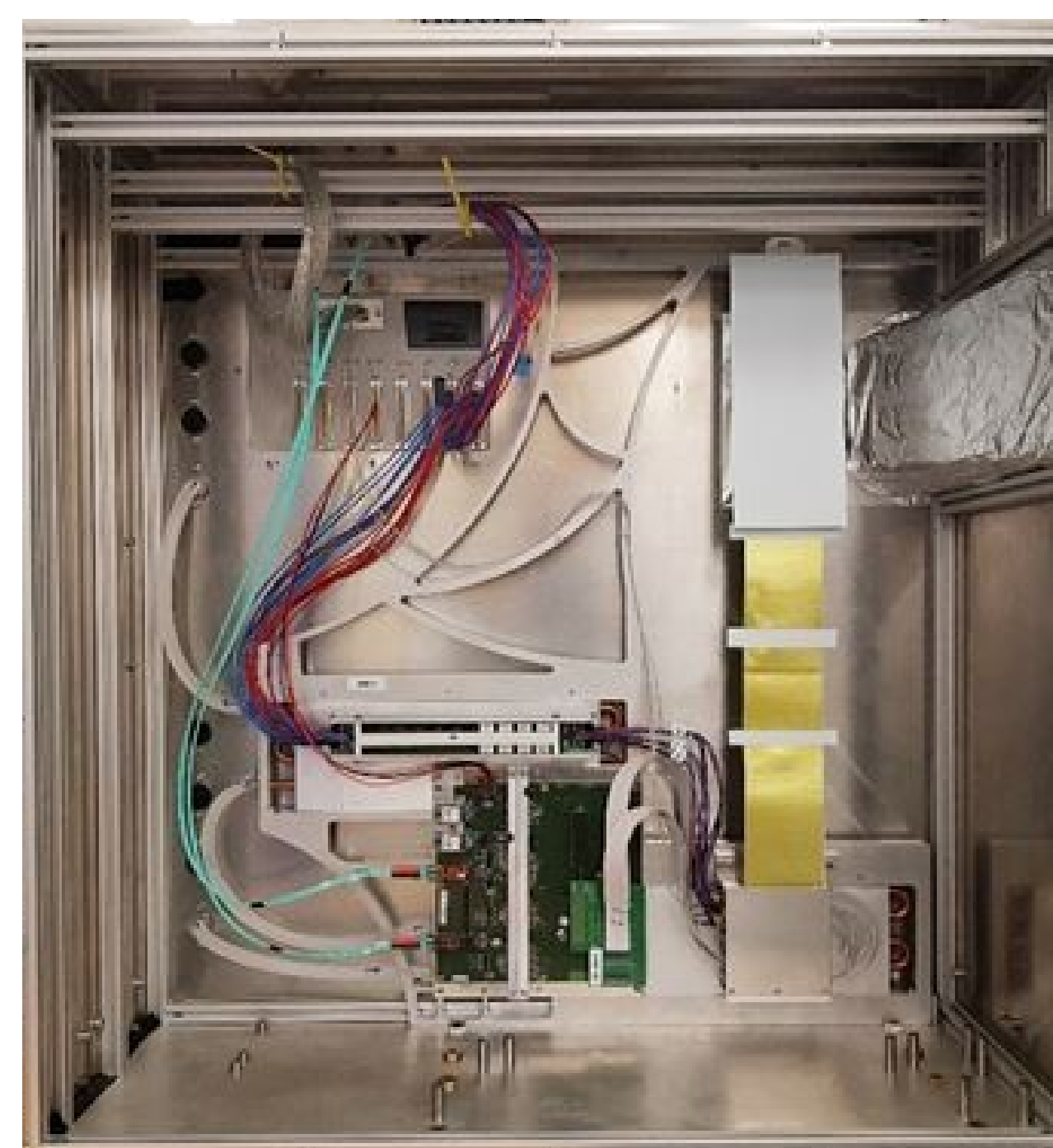
mSTS enclosure with ladder holding modules covered with shielding
