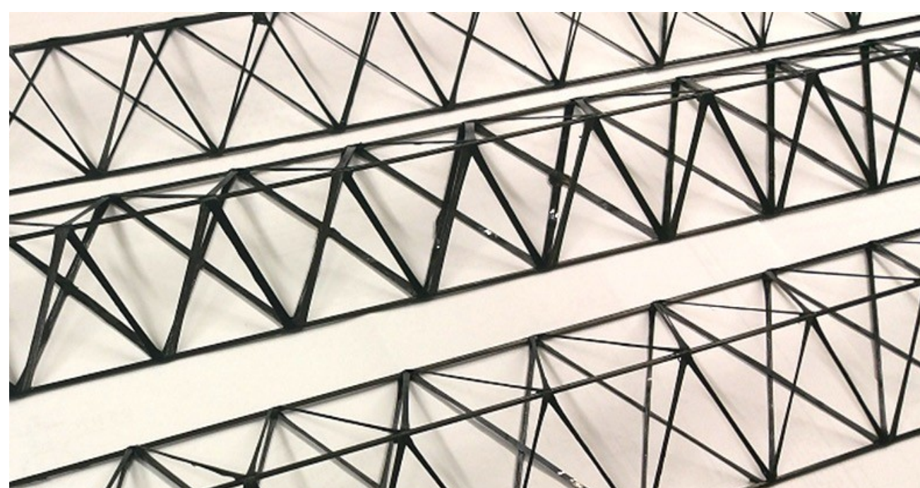
Carbon Fiber support structures produced with winding technique
