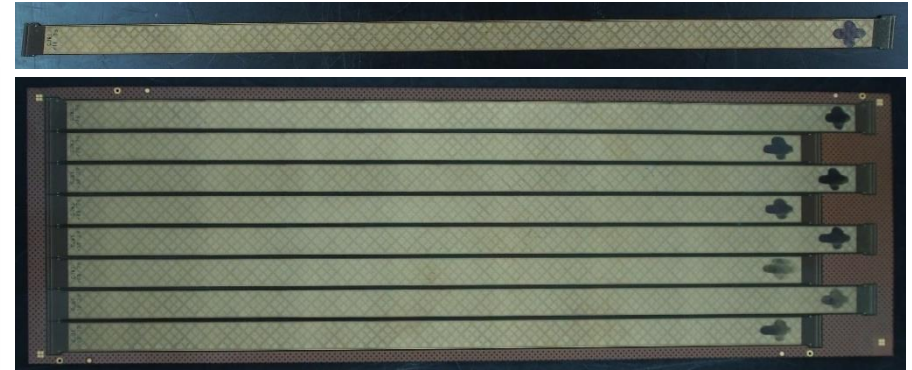
Low mass microcables with varying length. Top: single cable. Bottom: sheet of 8 cables.
