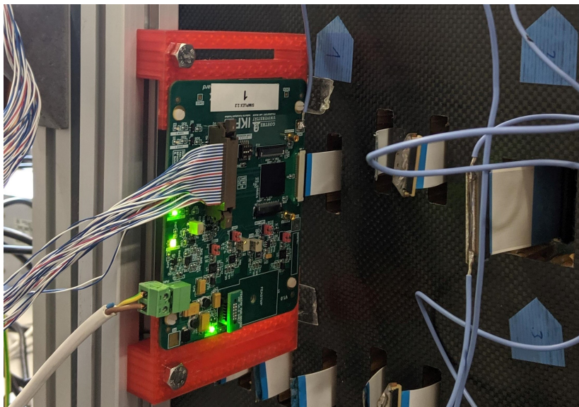
Figure 5.1: A SPADIC 2.2. connected to a small TRD chamber in the laboratory.
