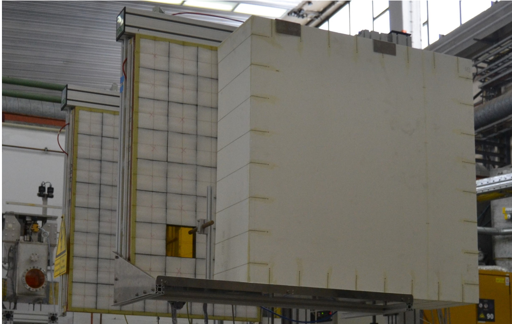
Figure 5.2: The two TRD chambers in the experimental setup. The chamber in the front was used in the measurements.
