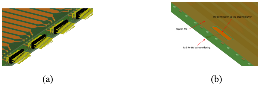
Fig. 4.4 (a) The signal transmission to the middle PCB and the connector to FEE. (b) The HV connection on the bottom PCB.
