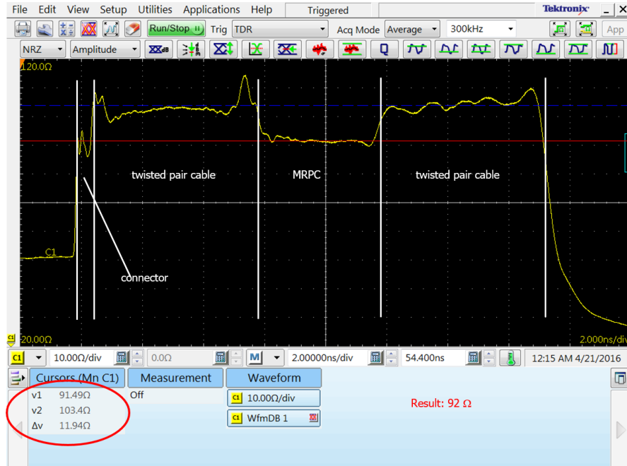
Fig. 3.21 The test results show that the characteristic impedance of the single-stack MRPC is 92 Ω.
