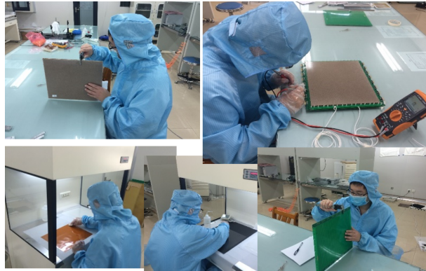
Fig. 4.9 Manufacturing MRPCs in the clean room and assembling MRPC on the clean desk.
