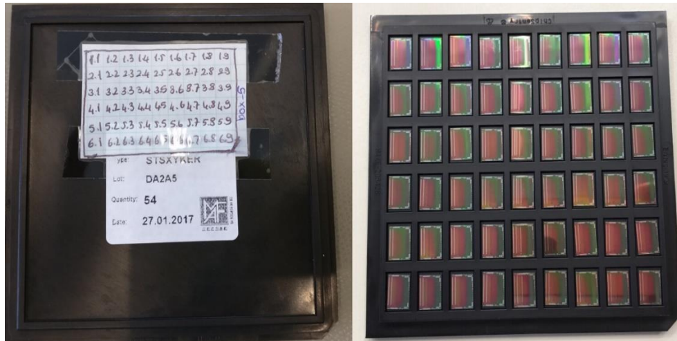
Figure 3.18: STS-MUCH/XYTER ASICs and the numbers given.
