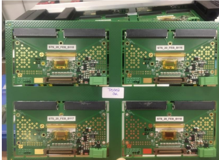
Figure 4.3: Prototype FEB-Bs with STS-XYTERv2 ASIC
