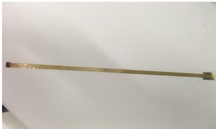
Figure 2.16: An example for the microcable with one ASIC.
