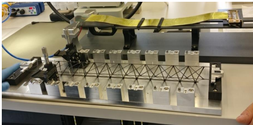
Figure 3.28: Tool that has been designed for the alignment of the modules to the ladders.
