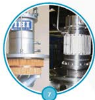
7 CRYOGENICS 2 new large 1.9 K helium refrigerators for HL-LHC near ATLAS and CMS
