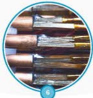
6 SUPERCONDUCTING LINKS Electrical transmission lines based on a high-temperature superconductor to carry current to the magnets from the new service galleries to the LHC tunnel.
