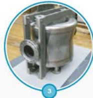
3 "CRAB" CAVITIES 8 superconducting "crab" cavities for each of the ATLAS and CMS experiments to tilt the beams before collisions.
