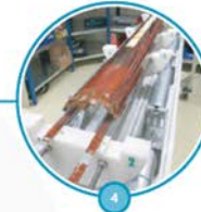
4 BENDING MAGNETS 2 pairs of shorter and more powerful dipole bending magnets to free up space for the new collimators.
