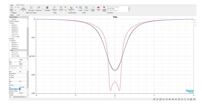
The simulation of magnetic fields Bx [T] along Z [m] for different X and Y
