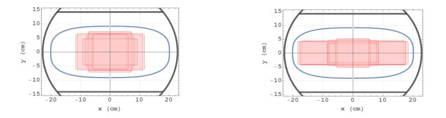
Approximately 400 x 200 mm of useful aperture and maximum beam size at different points along the CR arcs: pbar – left, ions – right (Figs from CDR of BPM - TYPE 1)
