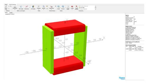
The simulation model of vertical steering magnet.
