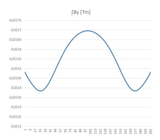
The simulation values of integral in the magnetic field By [T] for different points for the half circle with radius 0,1m.
