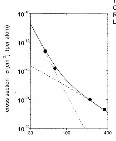
Theoretical total electron-capture cross sections for  $U^{92+}$  on a  $N_2$  target versus projectile energy (dotted line NRC, dashed line REC). The solid line refers to the sum of both predictions.
