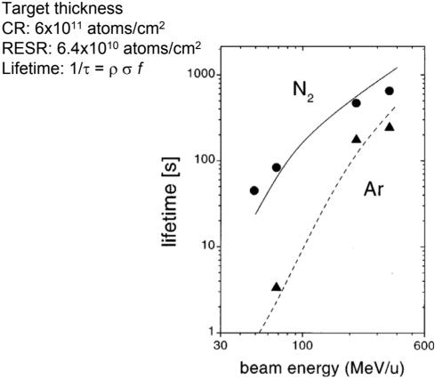
Experimental lifetimes for  $U^{92+}$ -ions obtained at the various beam energies for the case of a  $N_2$  (solid points) and an Ar (solid triangle) gaseous target (1x10<sup>12</sup> particles/cm<sup>2</sup>). The solid line and the dashed line (for the  $N_2$  and Ar target) represent theoretical lifetime estimates.
