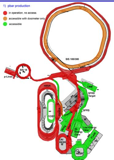
Protons from the p-Linac are injected into the SIS18 transported to the SIS 100 guided to the pbar-production target, accumulate and pre-cooled in the RESR/CR and finally injected into the HESR where for example experiments with the PANDA detector are performed.
