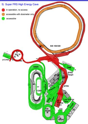
Primary beams are guided from the SIS 100 onto the target of the Super Fragment Separator. The cave for High Energy Nuclear Physics gets secondary beams from the Super Fragment Separator target area
