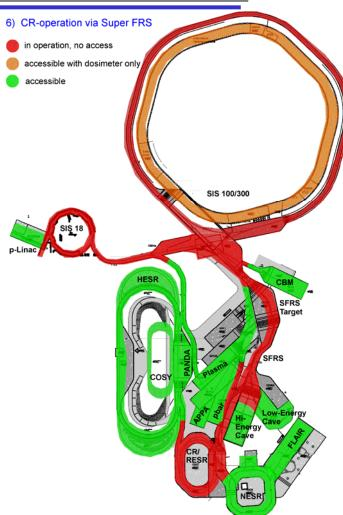
Primary beams from the SIS 100 are directed onto the target of the Super Fragment Separator. The primary beam is fragmented and separated secondary beams are guided through the Super Fragment Separator and injected into the CR.
