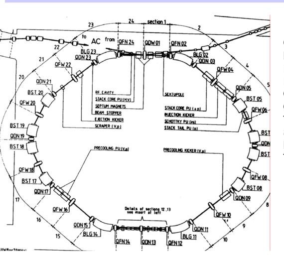
Circumference 156.5 m Max Rigidity 12 Tm Rev. frequency 1.85 MHz Rev. period 540 ns  $Q_{x}$ 2.26 2.26 Transition energy γ<sub>t</sub> 2.4 Slip factor n -0.106Momentum acceptance 6% Transverse acceptance 100 mm mrad
