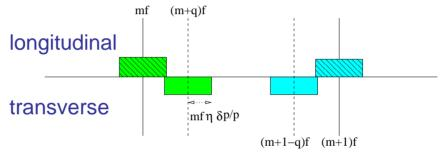
Overlap at upper band limit (2 GHz) for antiprotons  $\delta p/p \geq 8.7 \times 10^{-3}$  for RIBs  $\delta p/p \geq 3.6 \times 10^{-4}$   $\Rightarrow$  no heating for antiprotons
