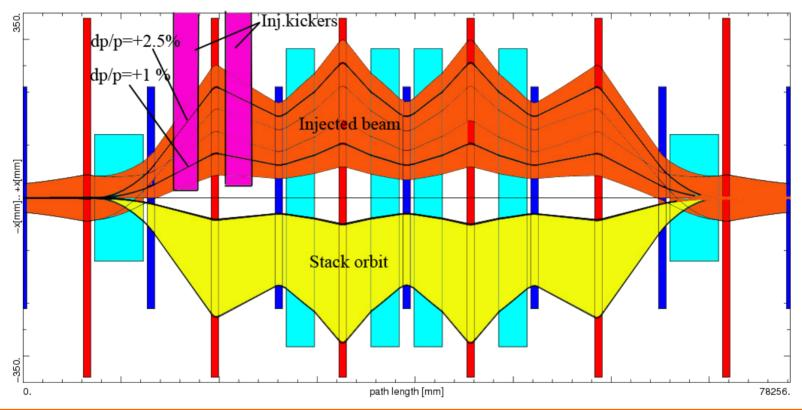
acceptance for injected antiproton beam (about half of the acceptance) : transverse  $\varepsilon_x$  =  $\varepsilon_v$  = 100 mm mrad, momentum spread = 1.5 %
