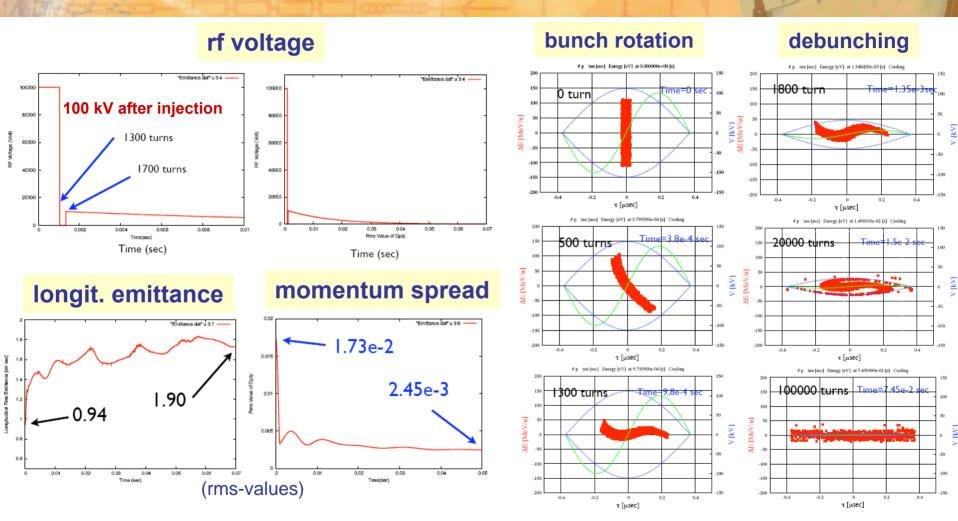
bunch rotation after injection of the short bunch (for both pbars and RIBs) reduces the momentum spread  $\Rightarrow$  reduction of cooling time
