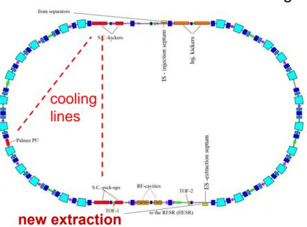
ring circumference and basic magnetic structure remain unchanged
