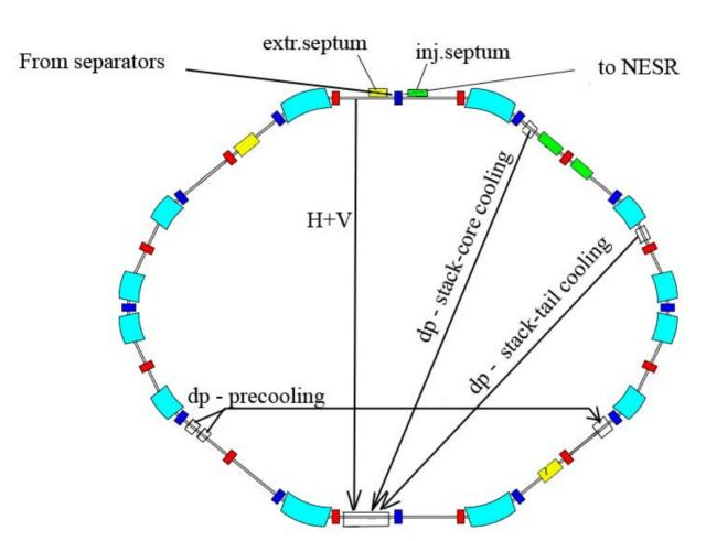
pre-cooling on injection orbit 0.8 - 2.4 GHz
