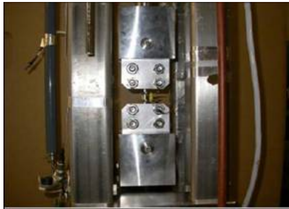
Figure 3.3: Test setup for the stress-strain measurement of the CuNi Tube
