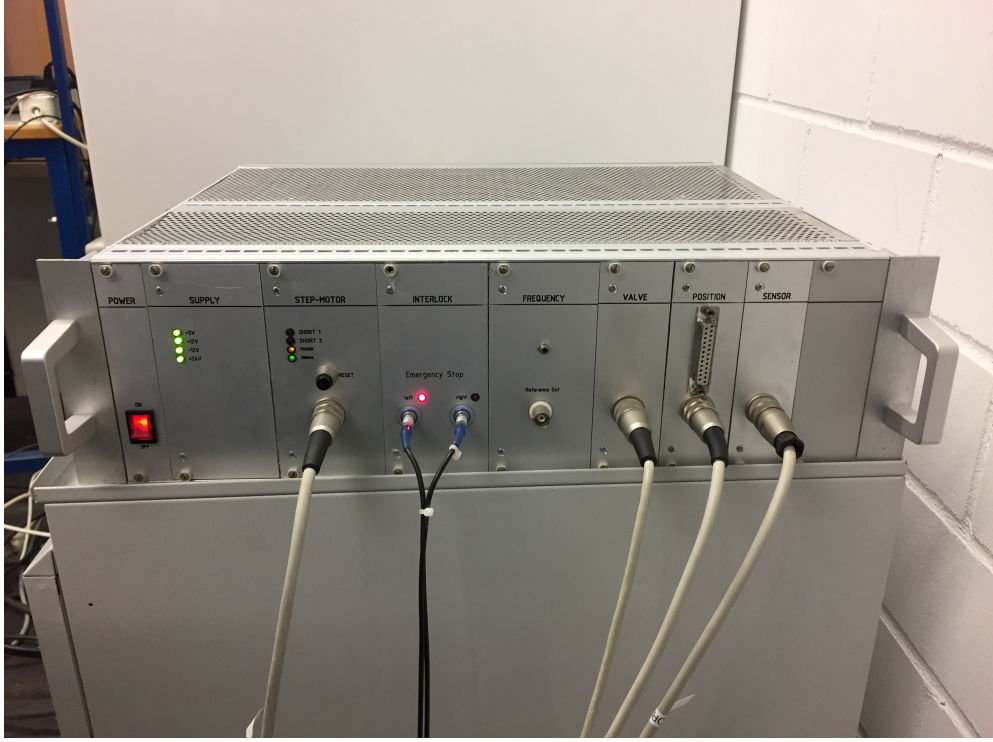
Figure 3.4: Photo of the electronics. On the front are the connections for the WTD and on the back the interface to the PC and the power supply.
