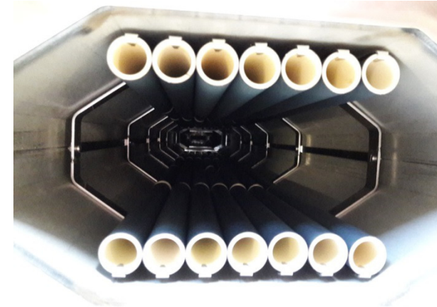
damping material to absorb rf signals travelling around the ring
