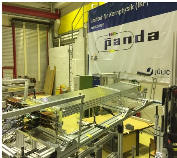
One of the two straw test systems. Beam enters from the right.
