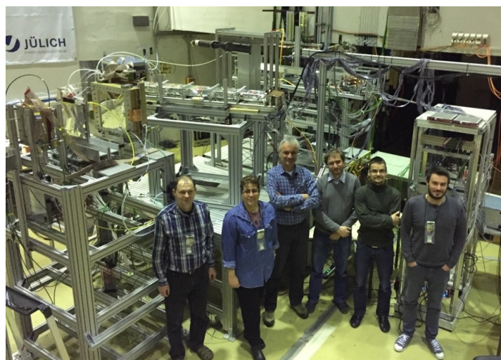
Test setups in new beam area. Beam from the back with ~2m beam line height.
