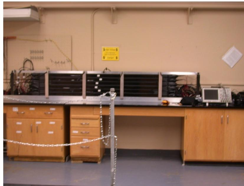
Resolution analyses were performed using the three-bar cosmic ray method. To speed-up the analysis process we run with six bars on top of each other and then select equidistant combinations of three bars for the analysis.
