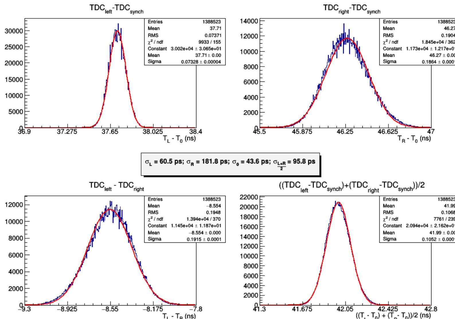
As is expectable the resolution for the PMT that closer to the measurement point is better than for another one.
