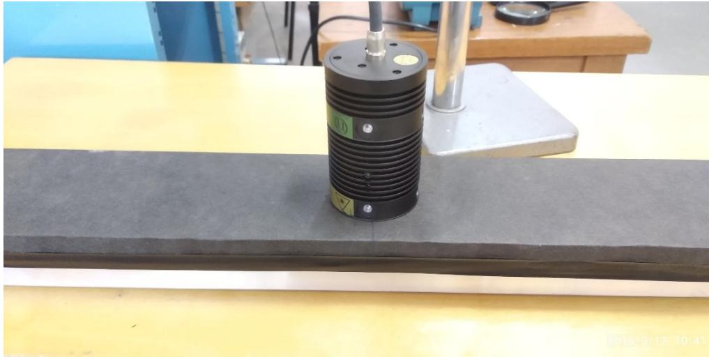
The laser head on top of the slap (central point).
