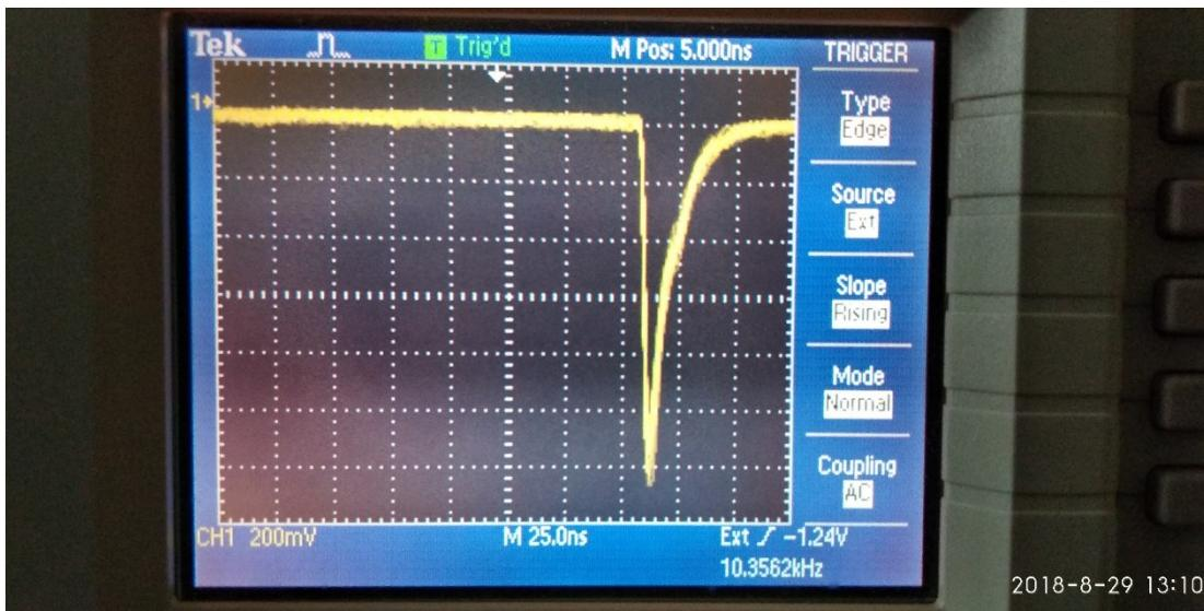
A screenshot of the signal from PMT 1 (R2083) from the laser set at the center of the slab.
