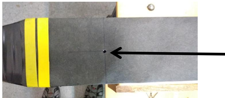
Three 5mm diameter holes in the wrapping materials were made along the slab. One in the center and one at a distance of 10 cm from each side.
