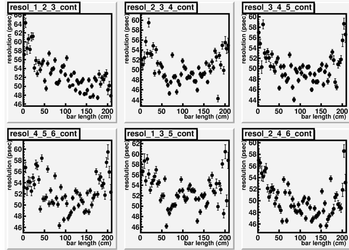
Parabola-like shape of the resolution vs position distributions looks similar to one obtained using laser measurements.
