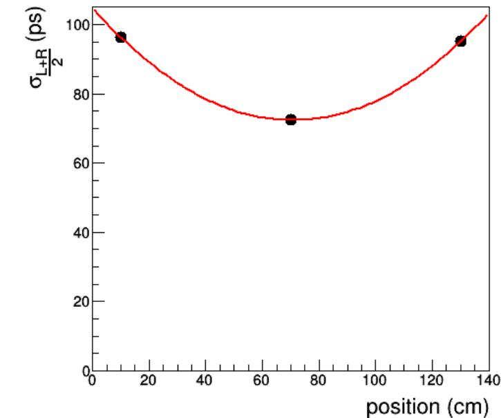
Expectable parabola-like shape for resolution vs position distribution.
