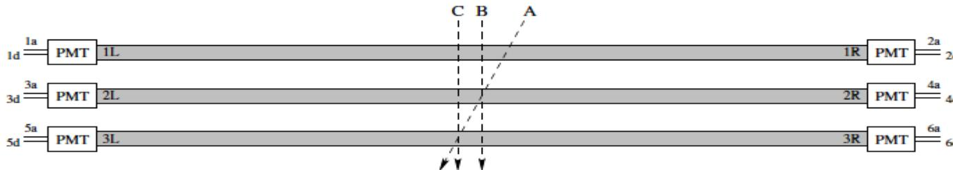
The time at which the particle interacts with  $i^{\text{th}}$  scintillator  $t_i = \frac{t_{iL}+t_{iR}}{2} - \frac{L}{2v_{\text{eff}}}$ , where  $t_{iL,R} = t_{\text{raw}} - t_{\text{ref}}$  with  $t_{\text{raw}}$  is the raw time reported by TDC and  $t_{\text{ref}}$  is the reference time.
