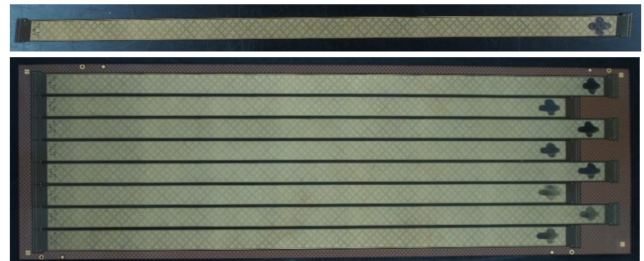
Low mass microcables with varying length. Top: single cable. Bottom: sheet of 8 cables. Pitch: 116 \mu\text{m}
