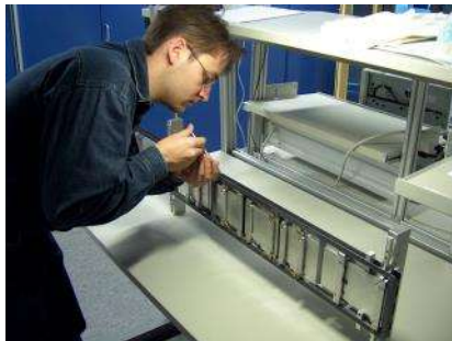
Manufacture of 700 carbon-fiber support structures for CMS Tracker, 2004-2005.
