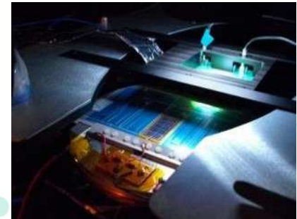
Quality Assurance of 250 silicon pixel detectors for CMS Tracker Upgrade, 2014-2016.
