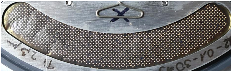
Lead nitrate (2.1 mg Pb) on Ti foil (2.3 \mu\text{m} ), tempered at 500°C for 30 min
