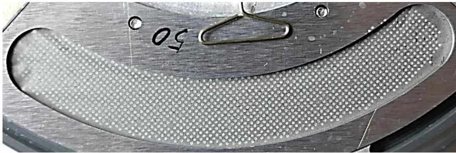
Lead nitrate (2.1 mg Pb) on carbon foil
