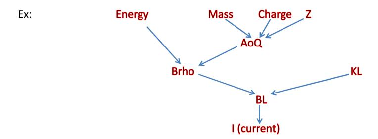
Machine model: parameter hierarchy for this machine (incl degraders etc...)
