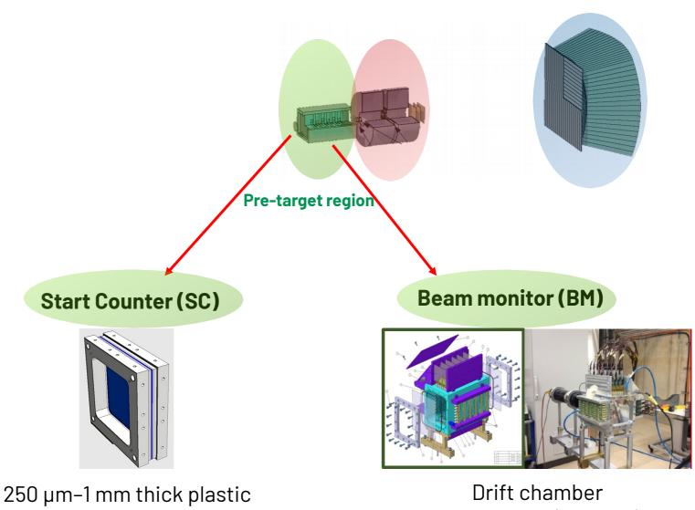
250 µm-1 mm thick plastic scintillator (depending on E beam)
