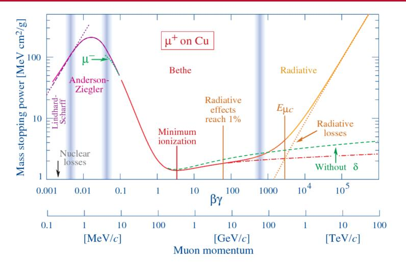
$$-\left\langle \frac{dE}{dx}\right\rangle = 2\pi N_a r_e^2 m_e c^2 \rho \frac{Z}{A} \frac{z^2}{\beta^2} \left[ ln \left( \frac{2m_e \gamma^2 v^2 W_{\rm max}}{I^2} \right) - 2\beta^2 - \delta - 2\frac{C}{Z} \right]$$
