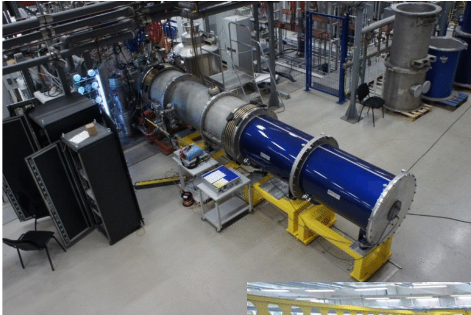
SIS100 quadrupole unit mounted in the test cryostat (blue) at JINR, Dubna
