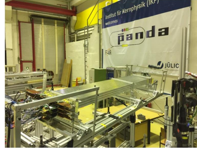
Straw testsystem for the ASIC/TRB readout. Beam from the right.
