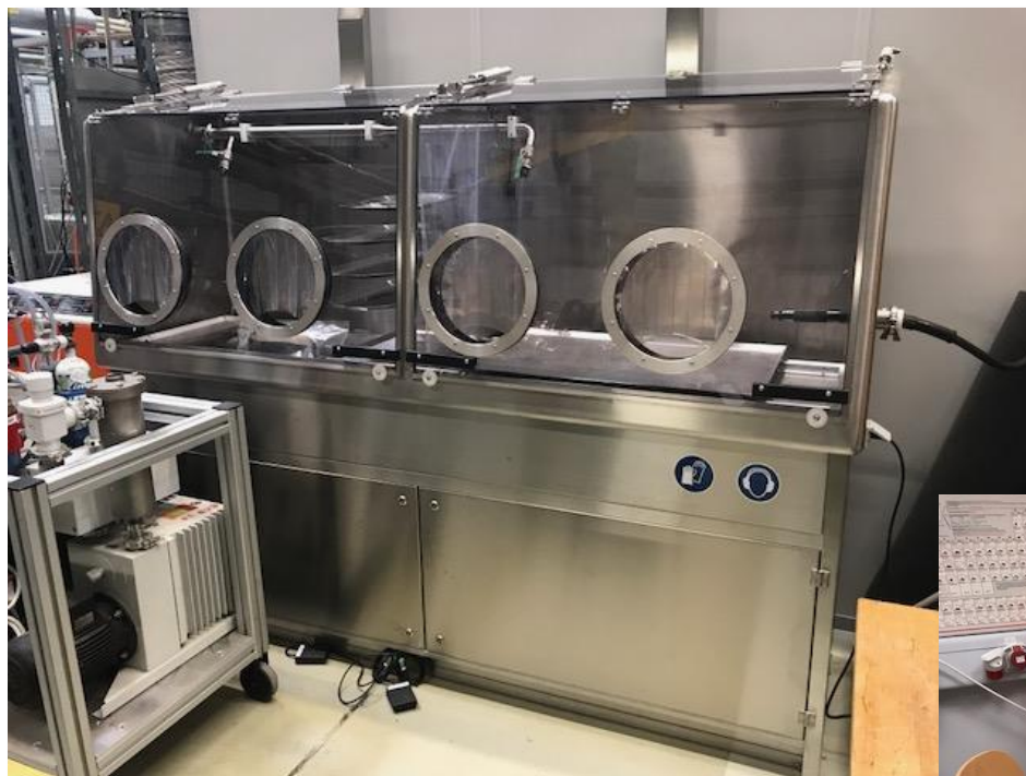
Glove box for service of heavy metal ion sources
