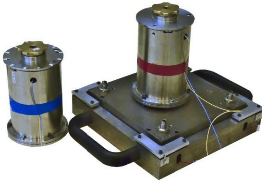
- LAPP active foot + LAPP sensors (one on ground used to monitor ground motion and 1 on top used in feedback) -
