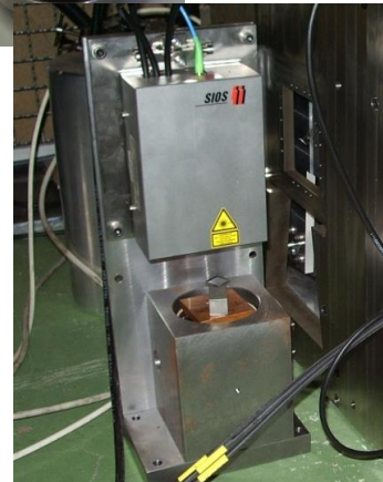
Vibrations sensors with interferometric measurement at CERN
