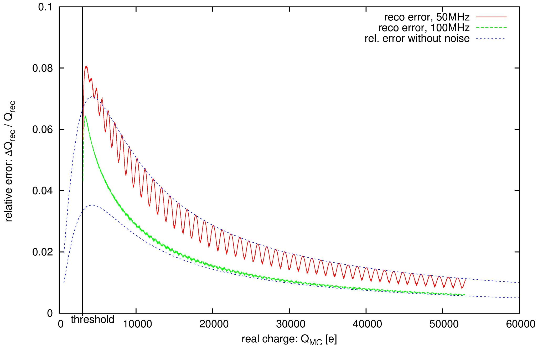
average relative error due to the clock for a reco Hit, protons[0..5] GeV/c, GEANT 4, clock: 50MHz
