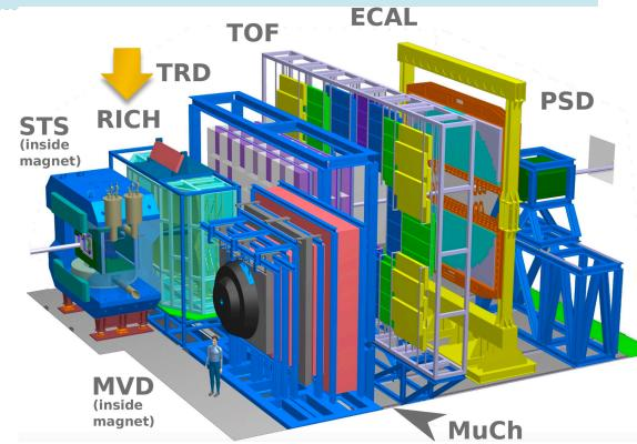
STS: tracking, momentum measurement, RICH+TRD: electron ID, TOF: hadron ID **ECAL**: photons, **PSD**: event characterization.
