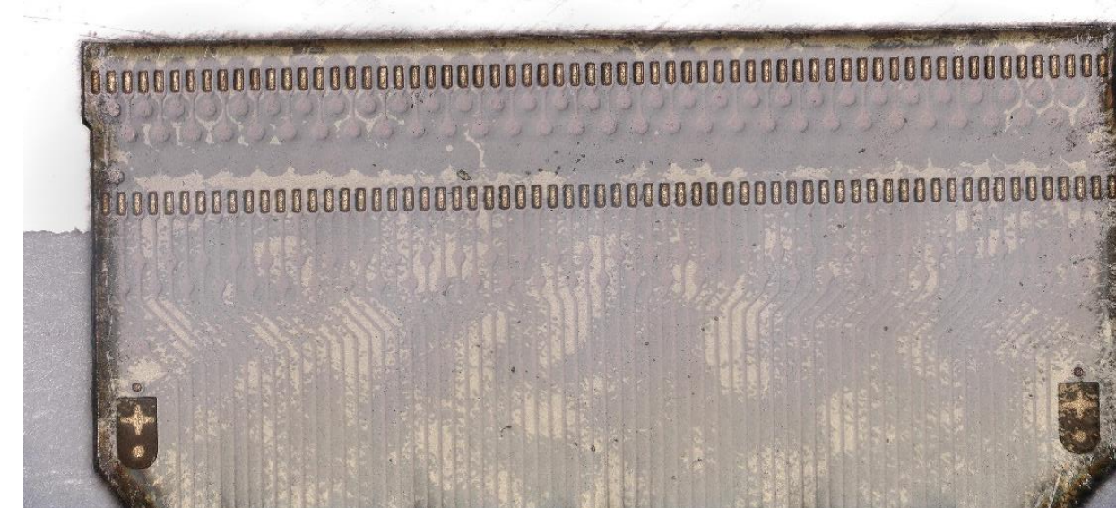
Close-up view on the head of the copper microcable. Two rows of 64 EPIG bond pads match the layout of the ASIC and the sensor. Fiducial marks are implemented for proper alignment during the bonding step.
