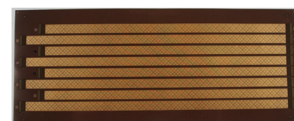
Sheet of 8 copper microcables as delivered by Dyconex.
