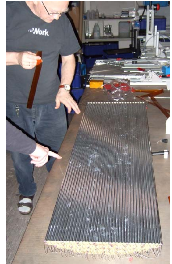
block of 6 straw layers glued together
